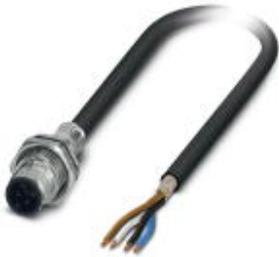
Flush-type plug, shielded, 4-pos., M12, A-coded, rear/screw mounting with M16 thread, with 2 m cable, 4 x 0.34 mm<sup>2</sup>
