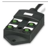
Sensor/actuator box, application: Standard, connection method: M12-SPEEDCON-socket Plastic, number of slots: 4, number of positions: 4, coding: A-coded, slot assignment: single, status display: yes, pnp; master cable connection: Fixed connection 180°, PUR/PVC, cable length: 10 m, shielding: no
