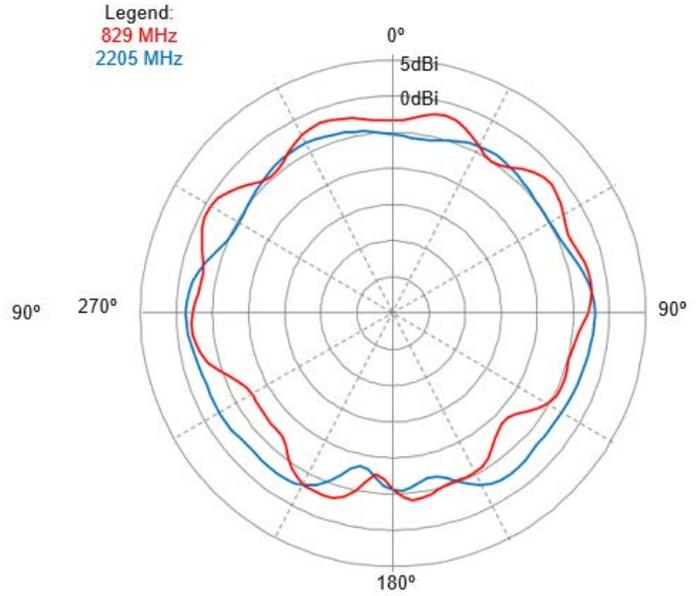
Data measured in free space and on plastic device enclosure
