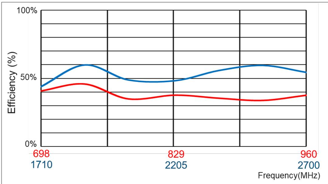
Data measured in free space and on plastic device enclosure
