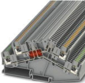
Disconnect terminal block, Double level with angled contour, one disconnect knife, and one disconnect point, Connection type: Push-in connection, Cross section: 0.14 mm<sup>2</sup> - 4 mm<sup>2</sup>, AWG: 26 - 12, Nominal current: 16 A, Nominal voltage: 400 V, Length: 127.5 mm, Width: 5.2 mm, Color: gray, Assembly: NS 35/7,5, NS 35/15
