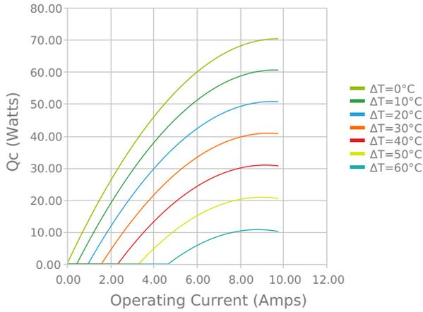
Heat Pumped at Cold Side
