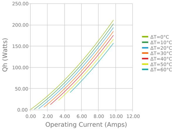
Total Heat Dissipated at Hot Side (Qh=Qc+Pin)
