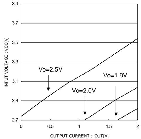
Fig.34 minimum input voltage in each output voltage
