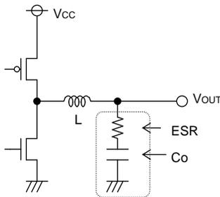
Fig.28 Output capacitor
