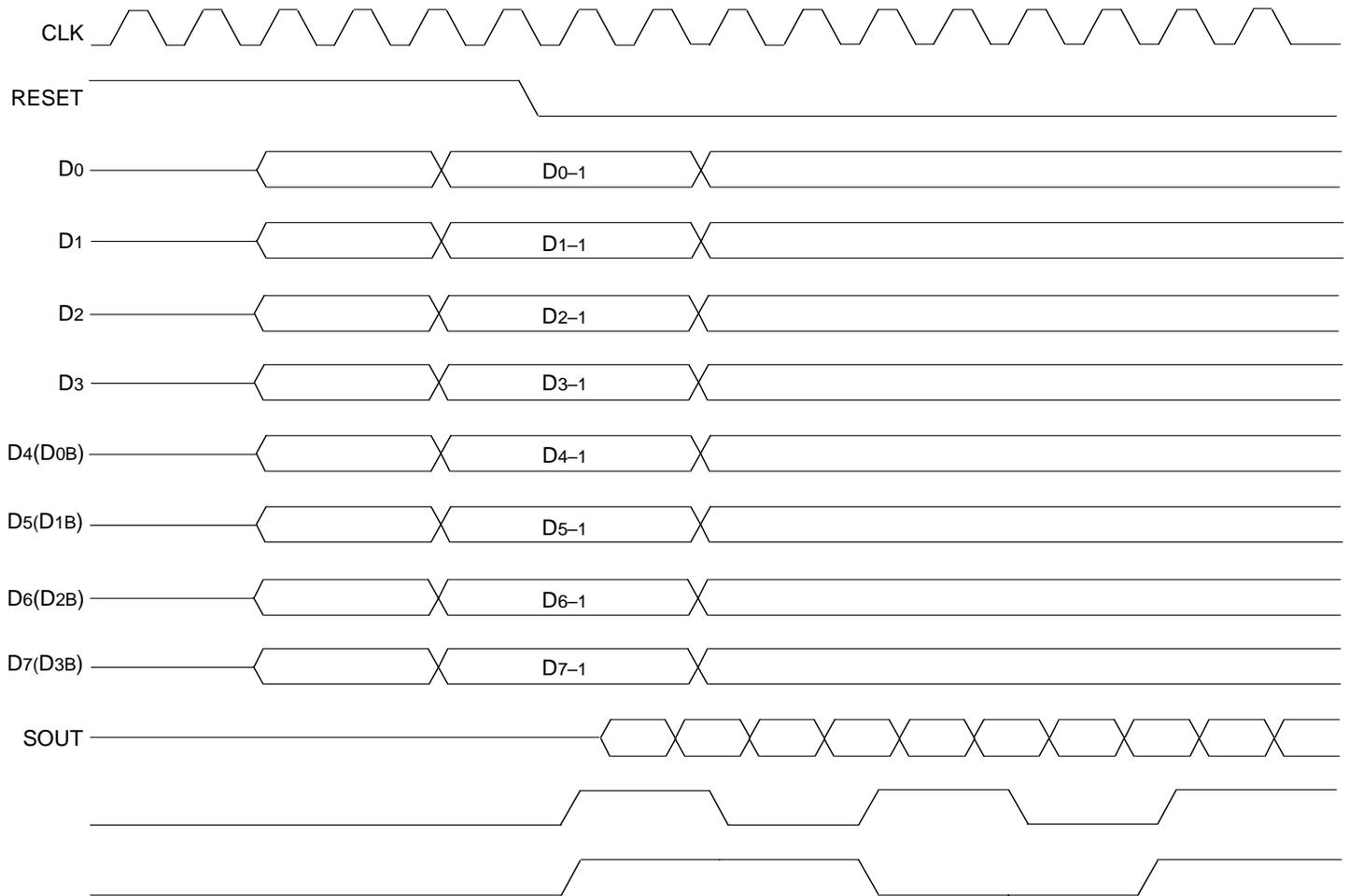
**Timing Diagram B. 8:1 Parallel-to-Serial Conversion**
