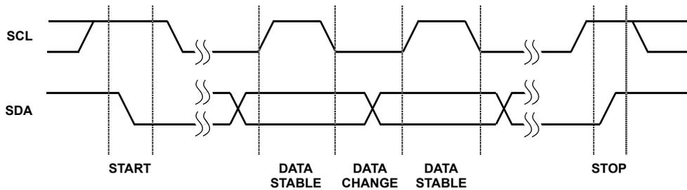
**FIGURE 17. VALID DATA CHANGES, START, AND STOP CONDITIONS**
