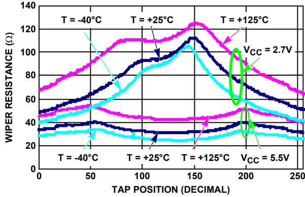
FIGURE 1. WIPER RESISTANCE vs TAP POSITION [I(RW) = V<sub>CC</sub>/R<sub>TOTAL</sub>] FOR 10kΩ (W)
