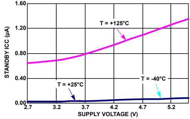
FIGURE 2. STANDBY I<sub>CC</sub> vs V<sub>CC</sub>
