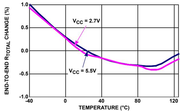
FIGURE 16. END-TO-END  $R_{TOTAL}$  % CHANGE vs TEMPERATURE, 50k (U)
