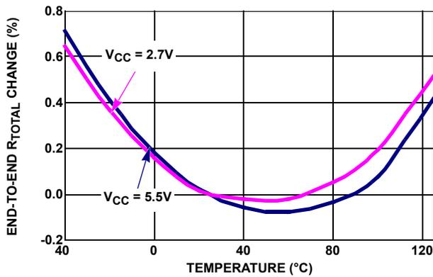
FIGURE 15. END-TO-END  $R_{TOTAL}$  % CHANGE vs TEMPERATURE, 10k (W)
