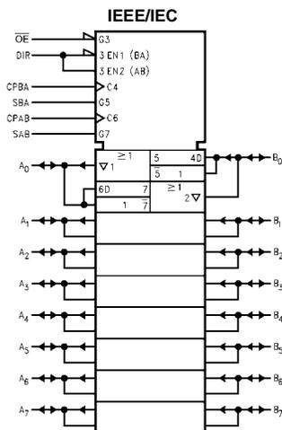
74LVTH646 Low Voltage Octal Transceiver/Register with 3-STATE Outputs
