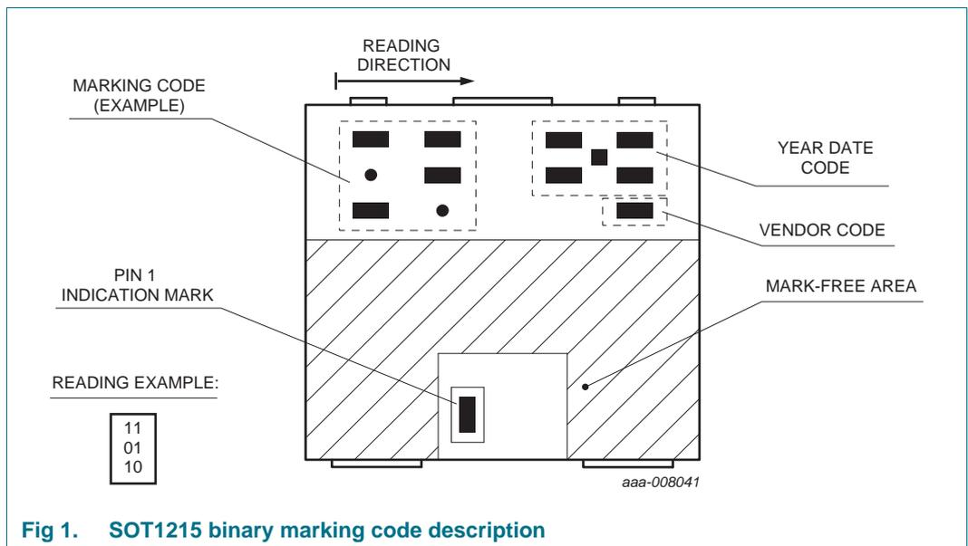
Fig 1. SOT1215 binary marking code description
