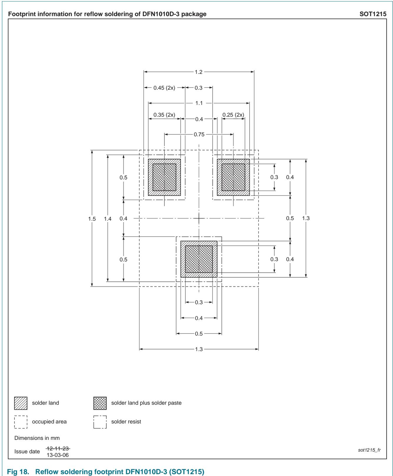
**Fig 18. Reflow soldering footprint DFN1010D-3 (SOT1215)**
