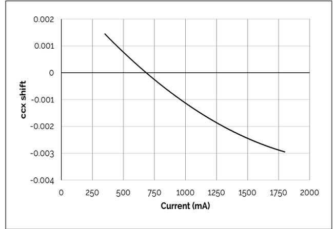
**Figure 9: V18B Drive Current vs. ccy Shift**
