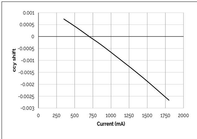
**Figure 10: V18C Drive Current vs. ccx Shift**
