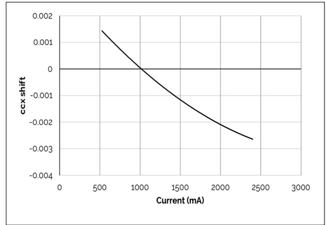
**Figure 11: V18C Drive Current vs. ccy Shift**
