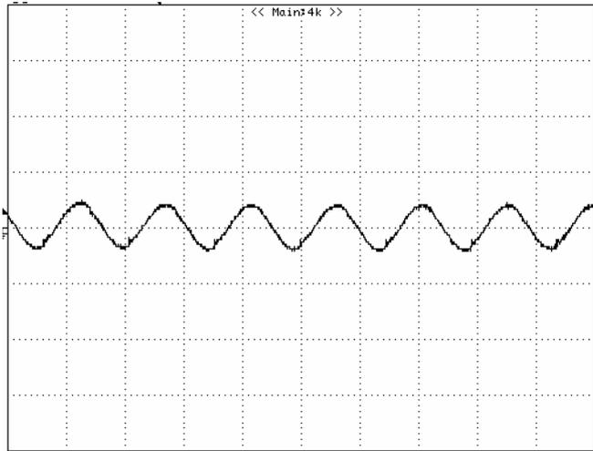
**Figure 11:** Input Terminal Ripple Current,  $i_c$ , at full rated output current and nominal input voltage with  $12\mu\text{H}$  source impedance and  $33\mu\text{F}$  electrolytic capacitor (100 mA/div, 2µs/div).
