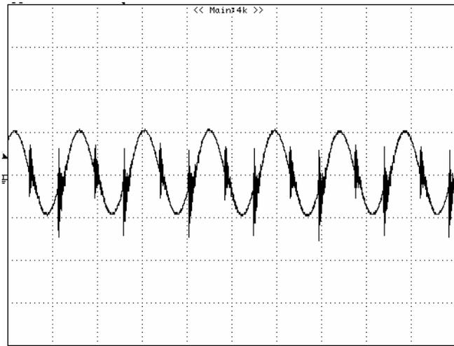
**Figure 14:** Output voltage ripple at nominal input voltage and rated load current ( $I_o=25A$ ) (20 mV/div, 2 us/div)
