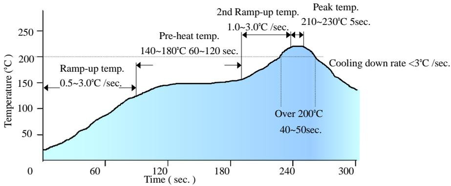
*Note: The temperature refers to the pin of E48SC, measured on the pin +Vout joint.*
