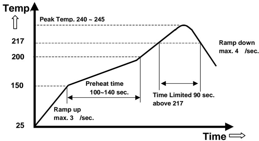
*Note: The temperature refers to the pin of E48SC, measured on the pin +Vout joint.*
