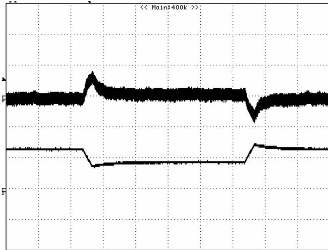
**Figure 8:** Output voltage response to step-change in load current (75%-50%-75% of  $I_o$ , max;  $di/dt = 0.1A/\mu s$ ). Load cap:  $10\mu F$ , tantalum capacitor and  $1\mu F$  ceramic capacitor. Top Trace:  $V_{out}$  (100mV/div, 200us/div), Bottom Trace:  $I_{out}$  (5A/div). Scope measurement should be made using a BNC cable (length shorter than 20 inches). Position the load between 51 mm to 76 mm (2 inches to 3 inches) from the module..
