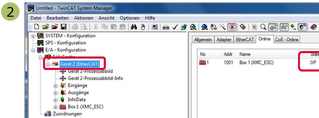
2 EtherCAT master view: Online status of master shows the slave in OP state. Cyclic counter is incrementing.
