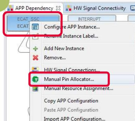
1 Right click on the ECAT\_SSC APP. From the context menu select „Manual Pin Allocator“ to open the pin allocation for the EtherCAT module.
