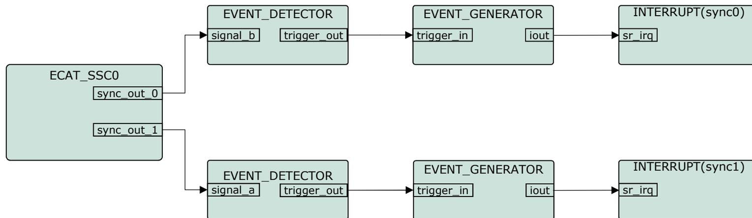
EVENT\_DETECTOR and EVENT\_GENERATOR APPs are instances of the event request unit (ERU) peripheral. Inside this example the ERU is used to propagate the signals sync0 and sync1 to the interrupt service routines.
