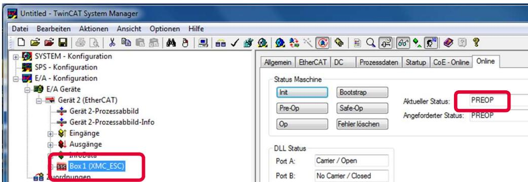
4 EtherCAT slave view: The PREOP-state of the slave is indicated within the TwinCAT system manager
