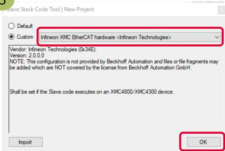
3 Select the Infineon device inside the drop down list and confirm with the OK button. Your project will be created.
