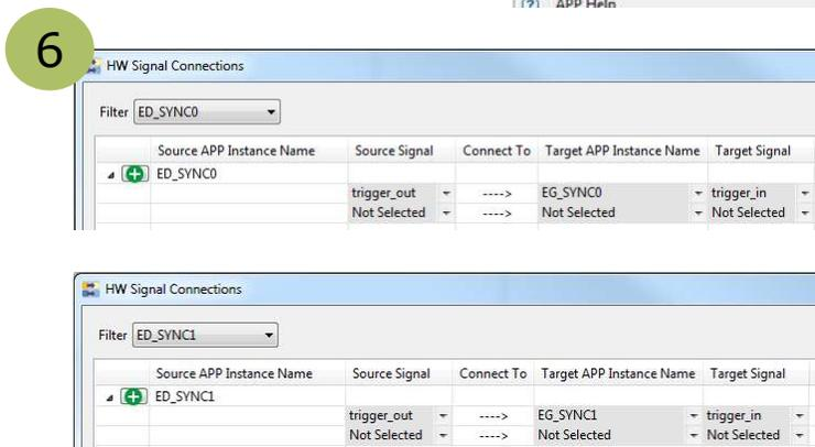
6 Connect the trigger\_out signals of the event detection units to the trigger\_in signals of the event generation units.
