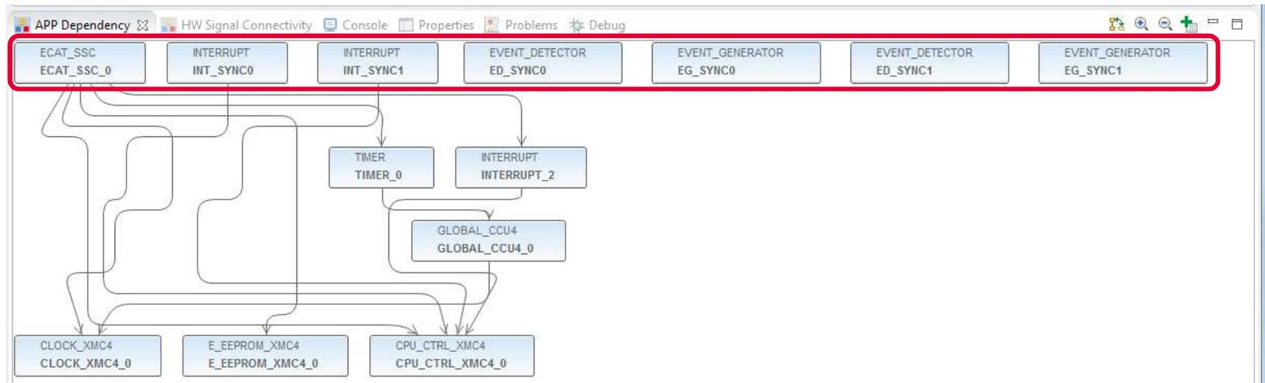
The ECAT\_SSC APP assigns the system resources (automatically done by DAVE by using the respective lower level apps) and pins (by manual configuration) to setup a proper EtherCAT communication. The EVENT\_DETECTOR, EVENT\_GENERATOR and INTERRUPT APPs are used inside this example to connect the sync\_out\_0 and sync\_out\_1 of the ECAT\_SSC APP to the interrupt service routines of the SSC-stack.
