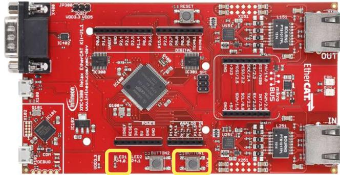
This example demonstrates the implementation of a EtherCAT slave node using the Beckhoff SSC tool to generate the slave stack code for „XMC4300 Relax EtherCAT Kit“
