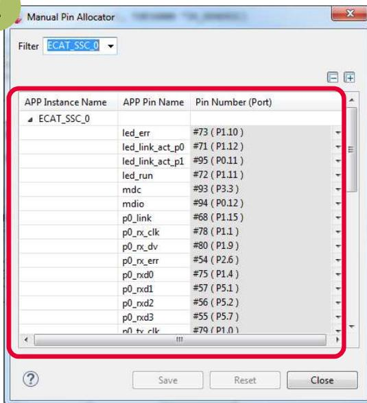
2 Inside Manual Pin Allocator you can configure the EtherCAT ports for your application. For the example provided, the configuration fits to the XMC4300 Relax EtherCAT Kit.
