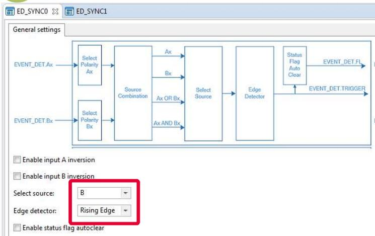
4 Select the respective source signal („A“ for SYNC0 and „B“ for SYNC1) and edge detection „Rising Edge“.
