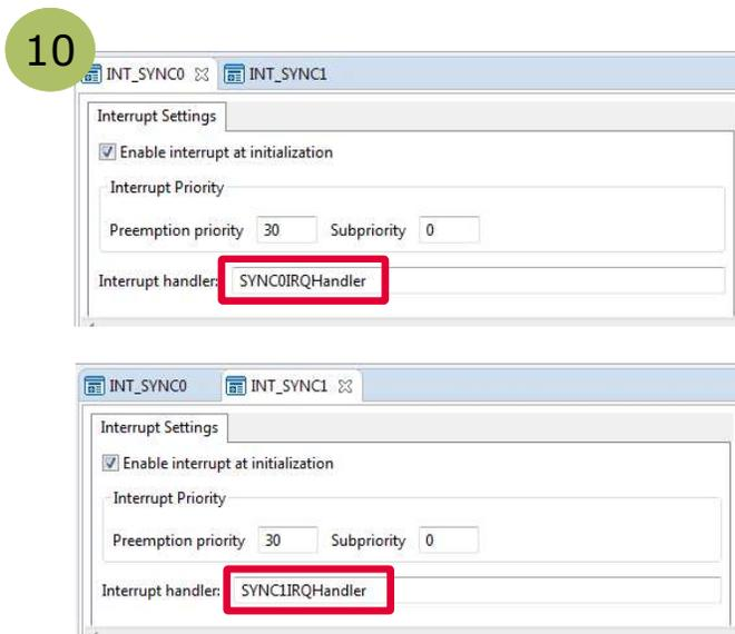
10 Set the interrupt service routine for sync0 and sync1 inside the configuration of the respective INTERRUPT APP.
