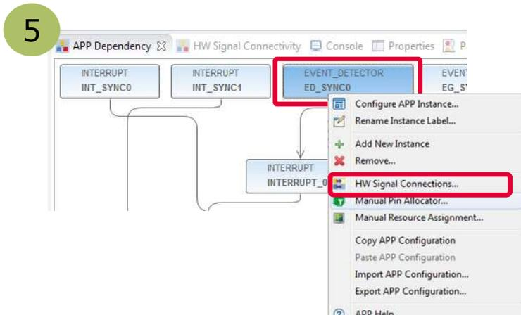
5 Right click on the EVENT\_DETECTOR APP for SYNC0 and SYNC1. From the context menu select „HW Signal Connections “ to open the HW Signal Connection dialog of the ECAT\_SSC APP.
