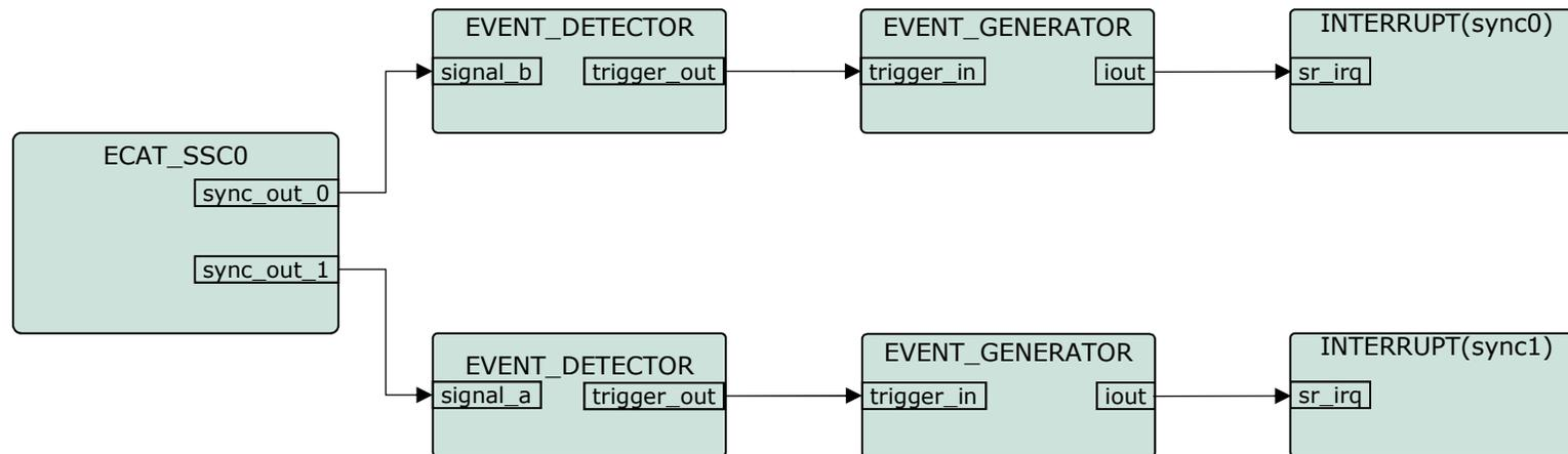
For distributed clock support, the sync0 and sync1 signals coming from the EtherCAT peripheral are used to trigger interrupts. Inside the interrupt service routines the respective API functions of the SSC protocol stack are called.
