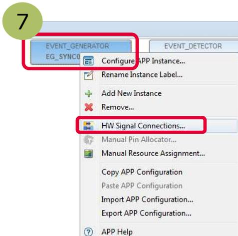
7 Right click on EVENT\_GENERATOR for sync0 and sync1. From the context menu select „HW Signal Connections “ to open the HW Signal Connection dialog of the EVENT\_GENERATOR APP.
