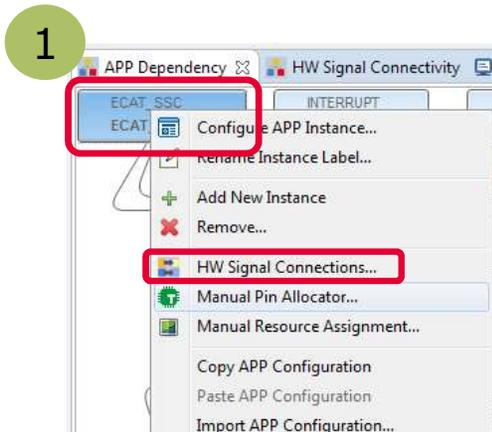
1 Right click on the ECAT\_SSC APP. From the context menu select „HW Signal Connections “ to open the HW Signal Connection dialog of the ECAT\_SSC APP.
