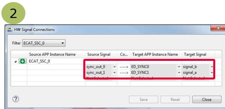
2 Connect the sync\_out\_0 and sync\_out\_1 signal to the a/b input of the event detection units .
