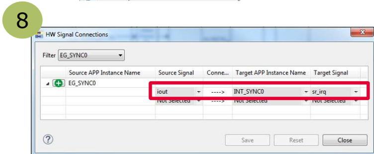
8 Connect the iout of the EVENT\_GENERATOR APP for sync0 to INTERRUPT APP of sync0. Proceed respectively for sync1.
