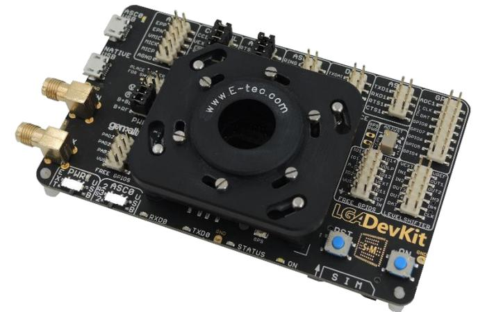
Socket solution for developing with **LGA** modules.
