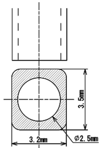
※ Nozzle with chamfering is recommended
