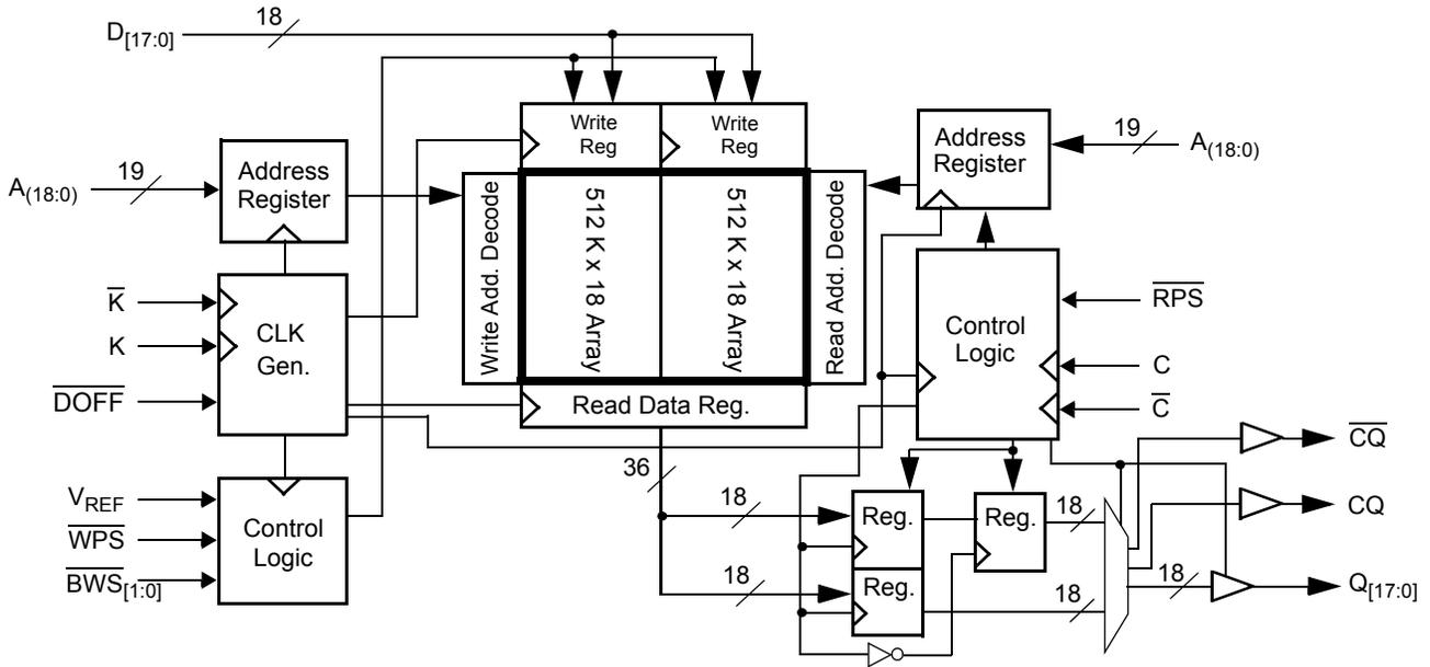
Logic Block Diagram – CY7C1314KV18
