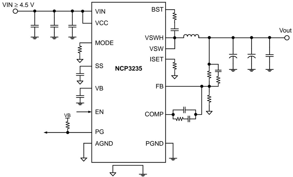
**Figure 2. NCP3235 Typical Application Circuit Without External VCC**
