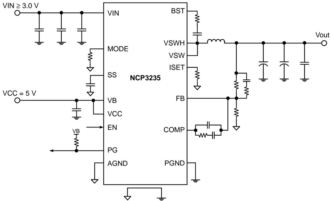
**Figure 3. NCP3235 Typical Application Circuit With VCC = 5 V**
