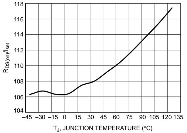
Figure 5. R<sub>DS(on)</sub>/I<sub>set</sub> vs. Temperature
