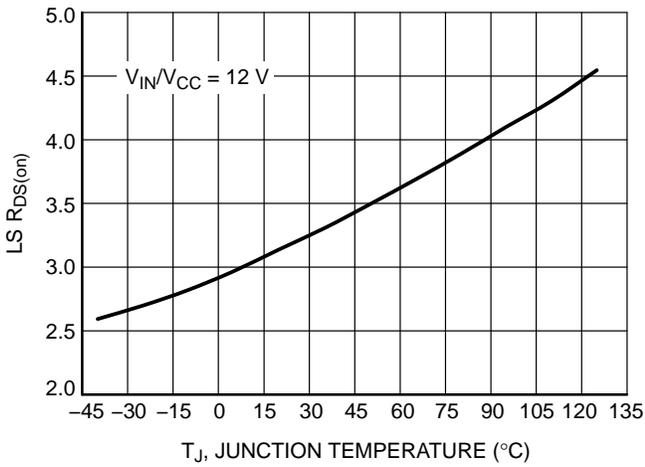
Figure 12. LS R<sub>DS(on)</sub> vs. Temperature
