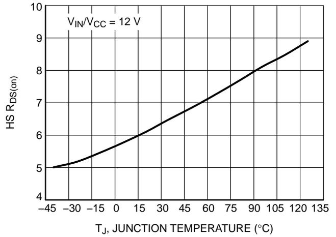
Figure 11. HS R<sub>DS(on)</sub> vs. Temperature
