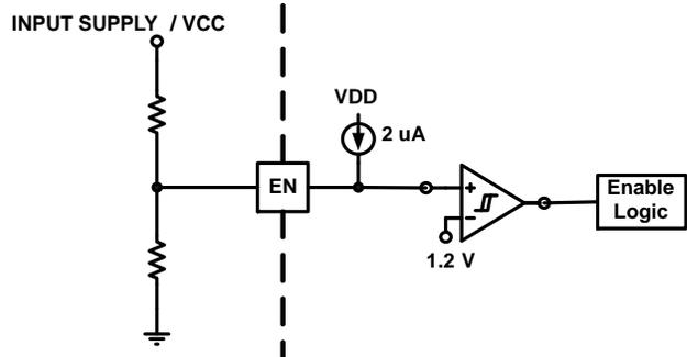
**Figure 28. Enable Functional Block Diagram**
