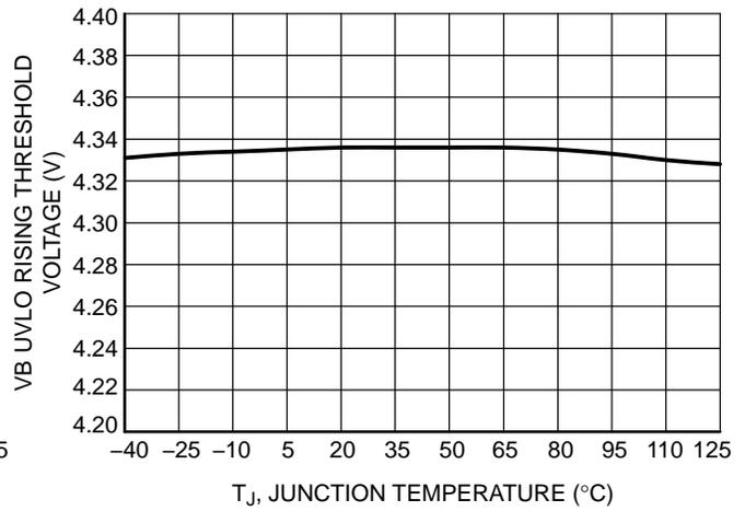
Figure 13. VB UVLO Rising Threshold vs. Junction Temperature
