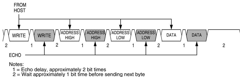
**Figure 19-15. Write Transaction**
