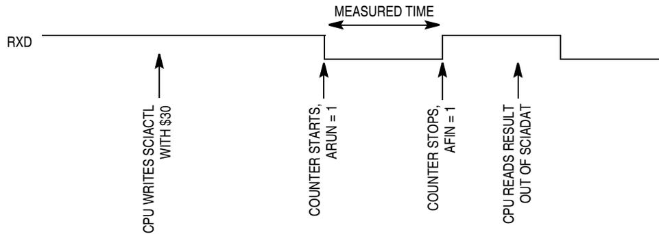
**Figure 13-23. Bit Time Measurement with ACLK = 1, Scenario B**
