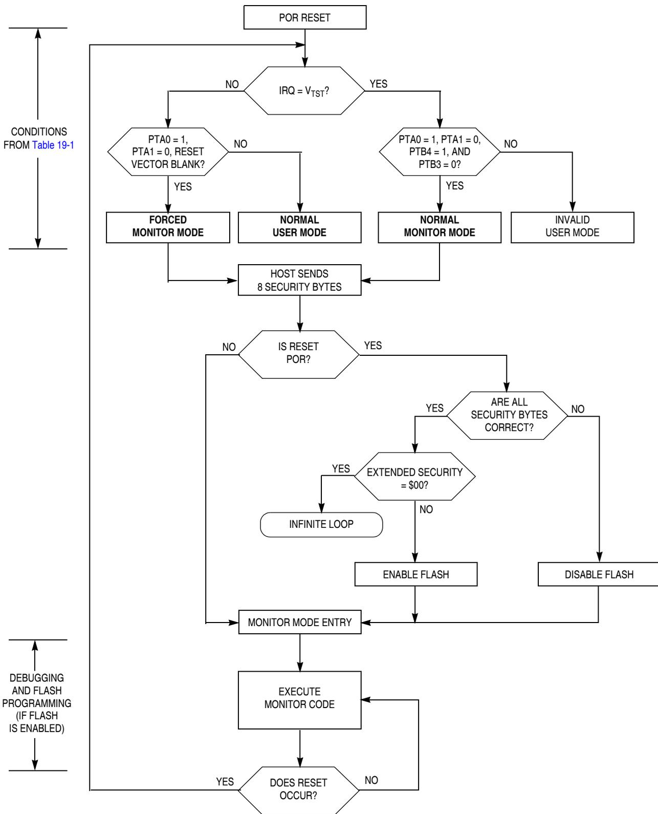
**Figure 19-8. Simplified Monitor Mode Entry Flowchart**
