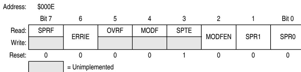
**Figure 15-13. SPI Status and Control Register (SPSCR)**
