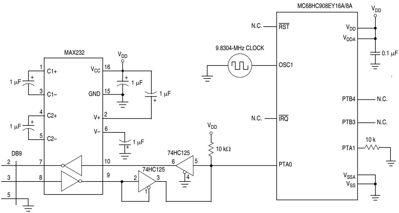
**Figure 19-10. Forced Monitor Mode ( $V_{\overline{IRQ}} = V_{DD}$ )**
