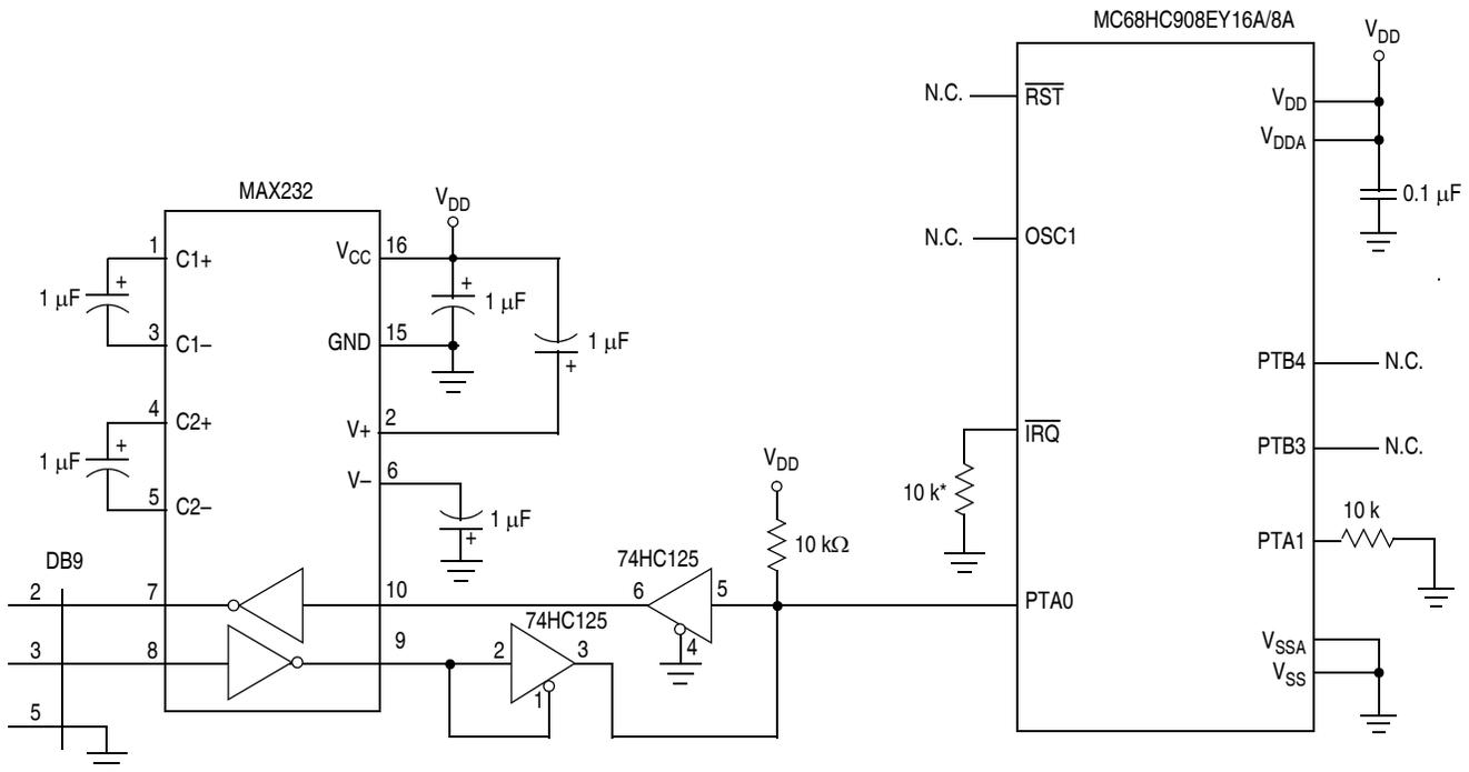
**Figure 19-11. Forced Monitor Mode ( $V_{\overline{IRQ}} = V_{SS}$ )**
