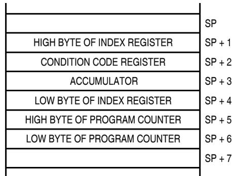
**Figure 19-16. Stack Pointer at Monitor Mode Entry**
