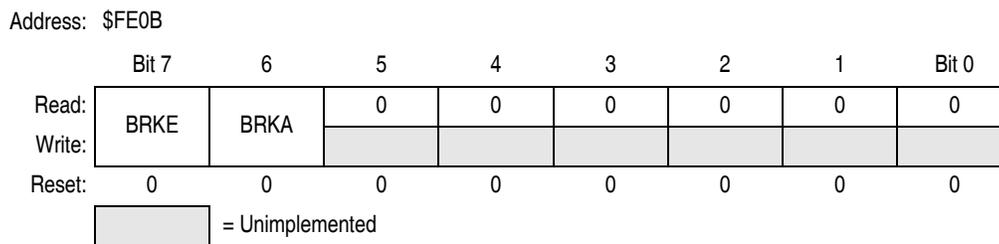
**Figure 19-3. Break Status and Control Register (BSCR)**
