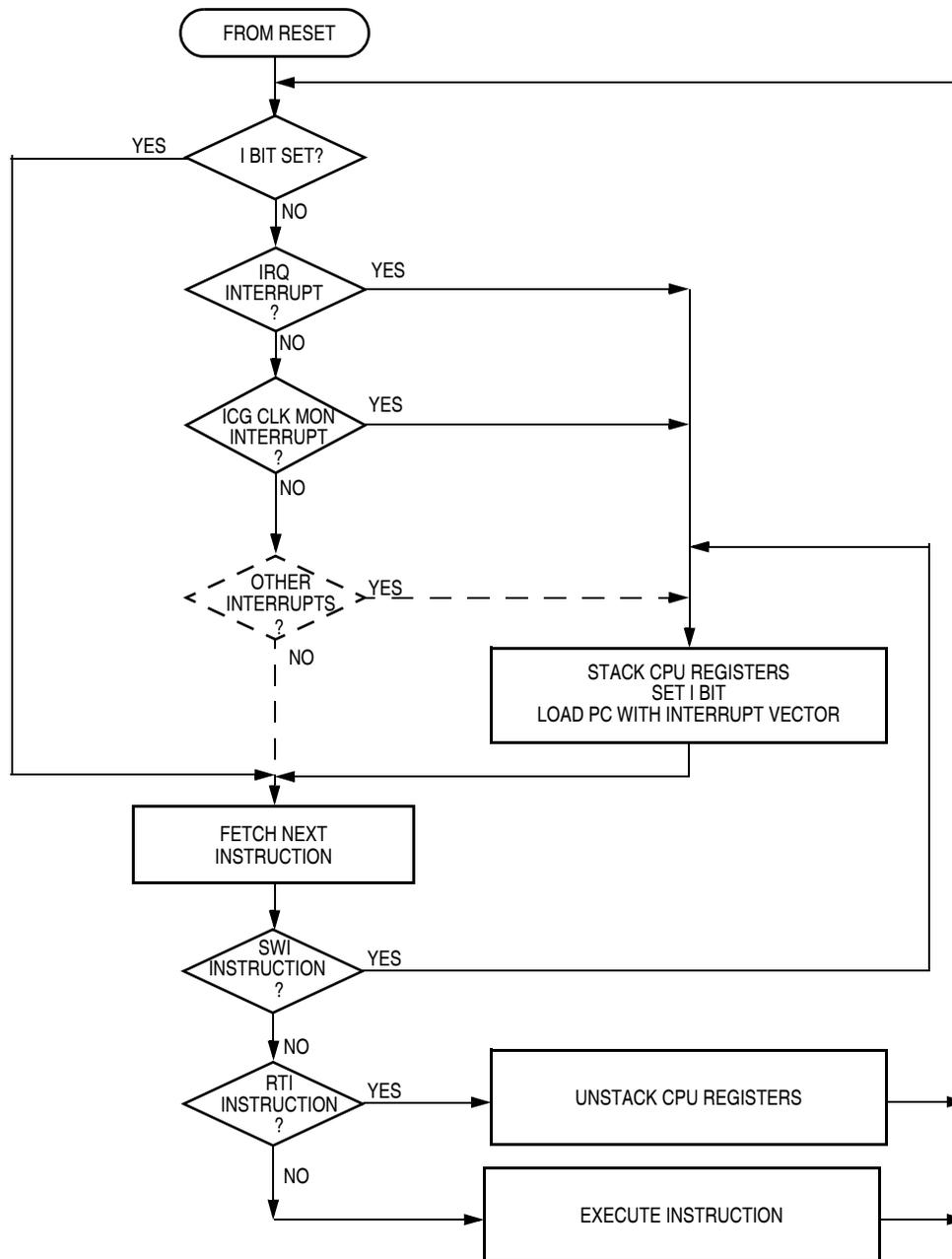
**Figure 14-9. Interrupt Processing**
