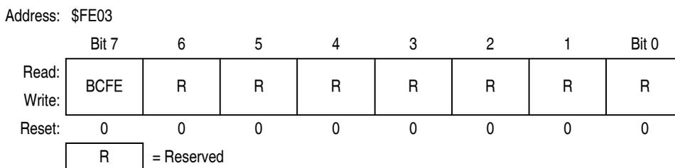
**Figure 14-21. SIM Break Flag Control Register (SBFCR)**
