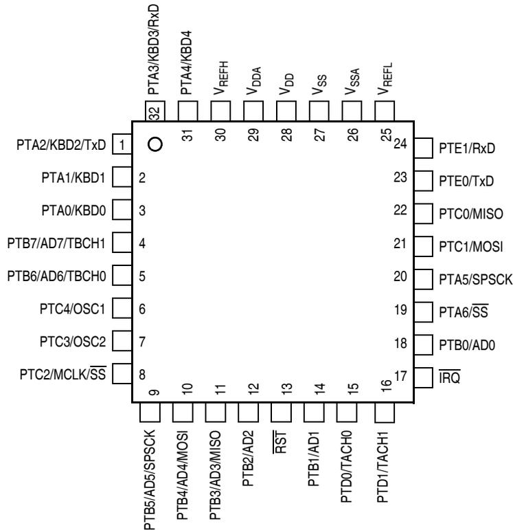
Figure 1-2. Pin Assignments
