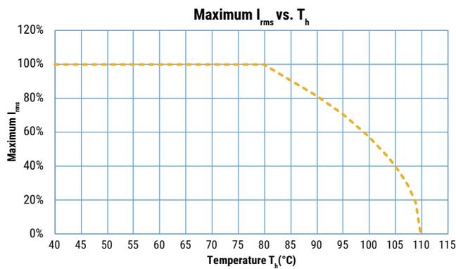
$T_h$  is the maximum ambient temperature surrounding the capacitor or hottest contact point (e.g. tracks), whichever is higher, in the worst operation conditions in °C.
