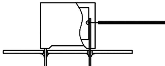
*Temperature monitored inside the capacitor.*
