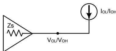
**AC Output Test Configuration**
