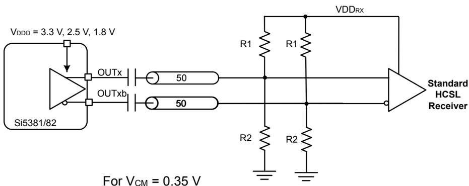
For  $V_{CM} = 0.35\text{ V}$
