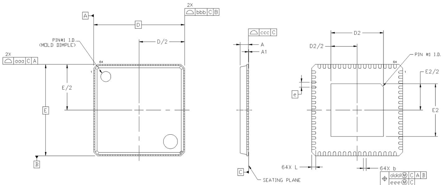
Figure 10.1. Si5381/82 9x9 mm 64-QFN Package Diagram
