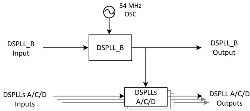
**Figure 3.1. High-frequency DSPLL**
