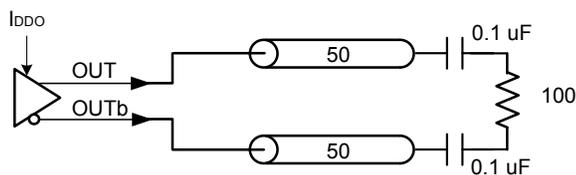
**LVCMOS Output Test Configuration**
