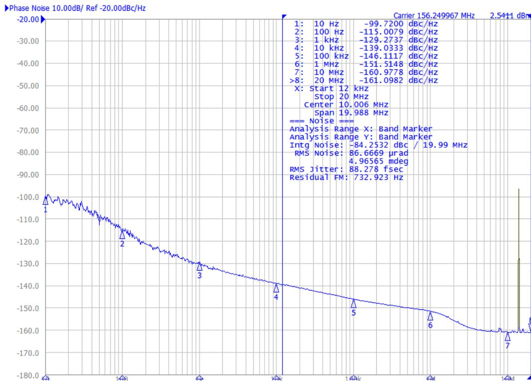
Figure 8.2.  $f_{IN} = 156.25\text{ MHz}$ ,  $f_{OUT} = 156.25\text{ MHz}$
