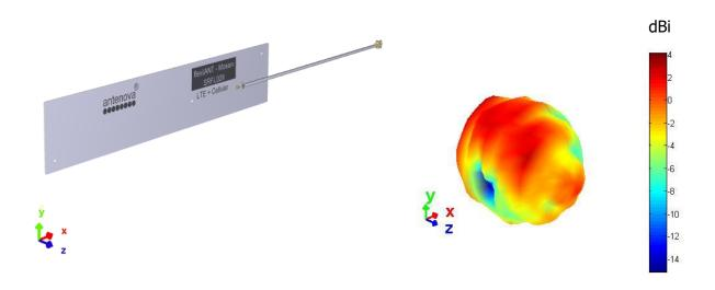
**3D pattern at 1990 MHz**Drag to rotate pattern and PCB by using Adobe Reader
