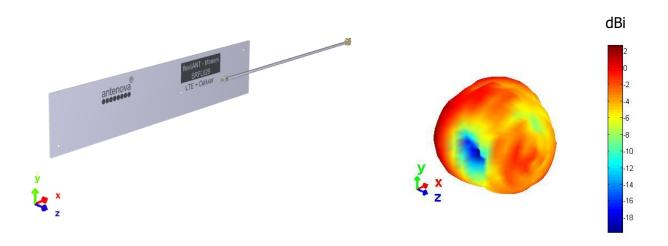
**3D pattern at 890 MHz**Drag to rotate pattern and PCB by using Adobe Reader
