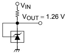
Shunt regulator ( $V_{KA} > V_{REF}$ )
