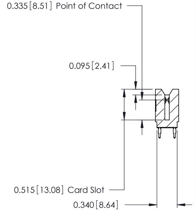
746 Series Ultra-Mate Card Edge Connector - Press Fit
