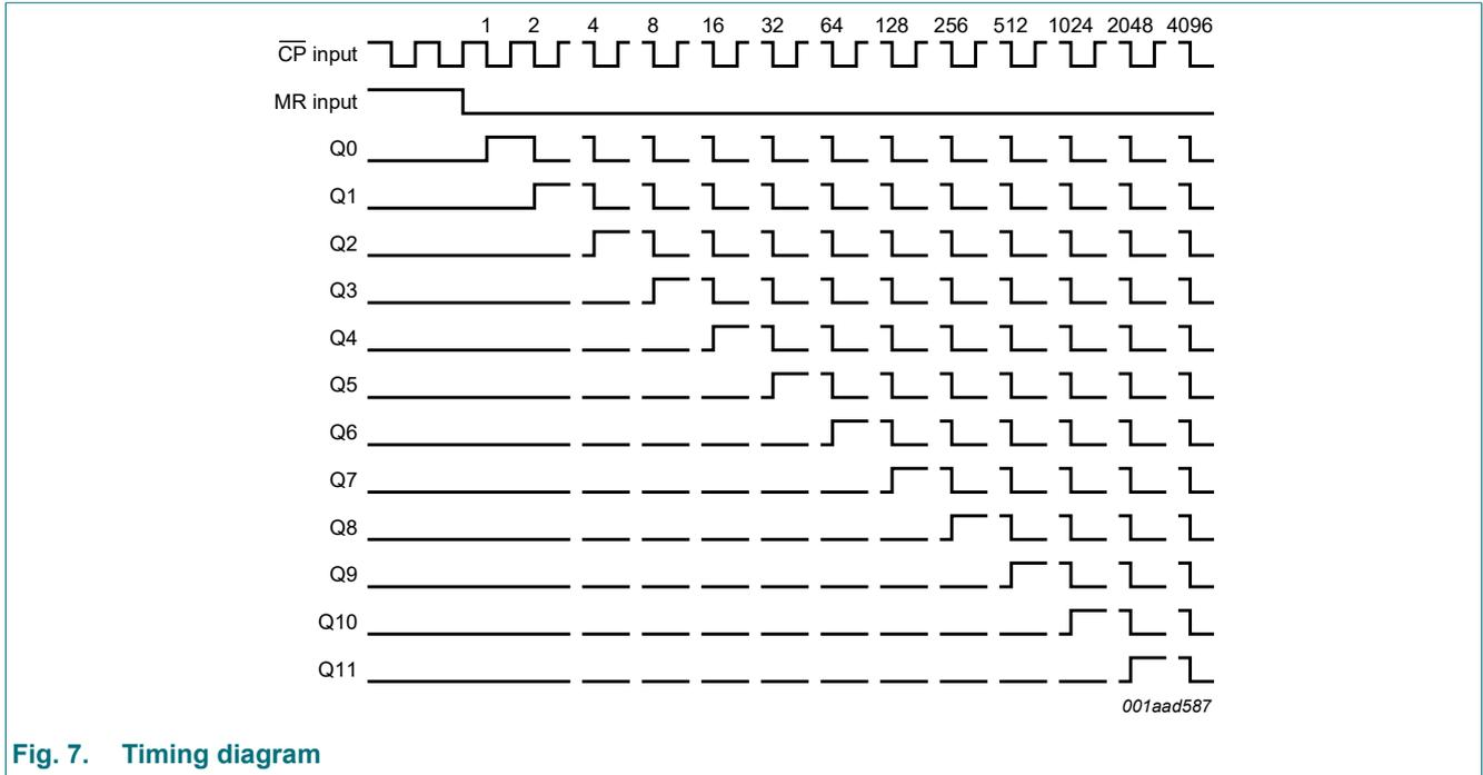
Fig. 7. Timing diagram
