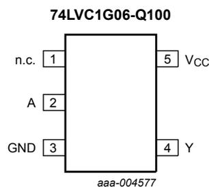
Figure 4. Pin configuration SOT353-1 (TSSOP5) and SOT753 (SC-74A)
