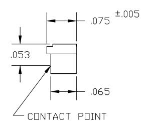
MATERIAL: HOUSING: GLASS FILLED THERMOPLASTIC, UL 94V-0, BLACK- 260°C PROCESS TEMP.
