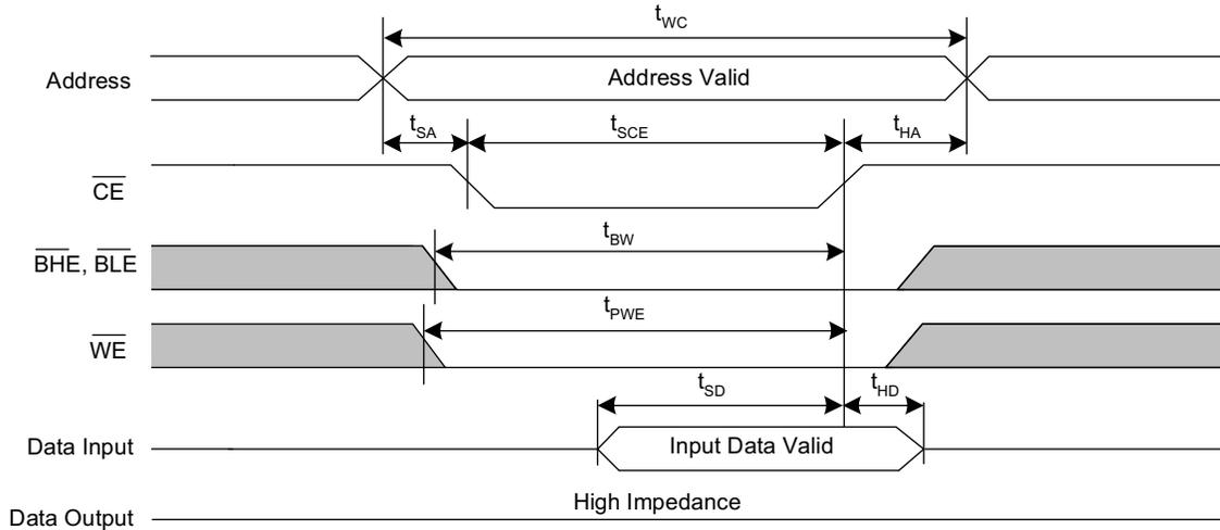
Figure 12. SRAM Write Cycle 3 ( $\overline{BHE}$  and  $\overline{BLE}$  Controlled) [36, 37, 38, 39, 40]
