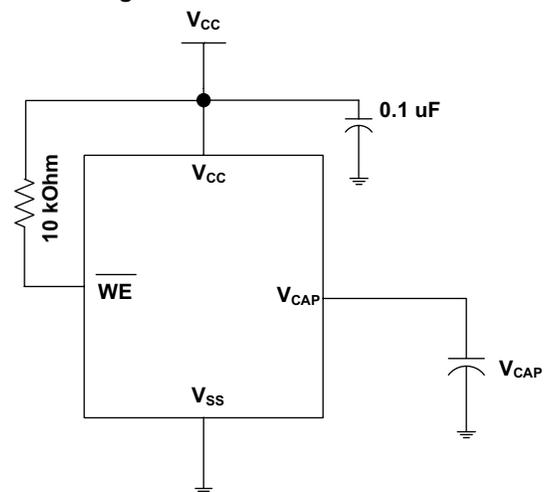
Figure 2 on page 4 shows the proper connection of the storage capacitor (V<sub>CAP</sub>) for automatic STORE operation. Refer to [DC Electrical Characteristics on page 16](#) for the size of the V<sub>CAP</sub>. The voltage on the V<sub>CAP</sub> pin is driven to V<sub>CC</sub> by a regulator on the
