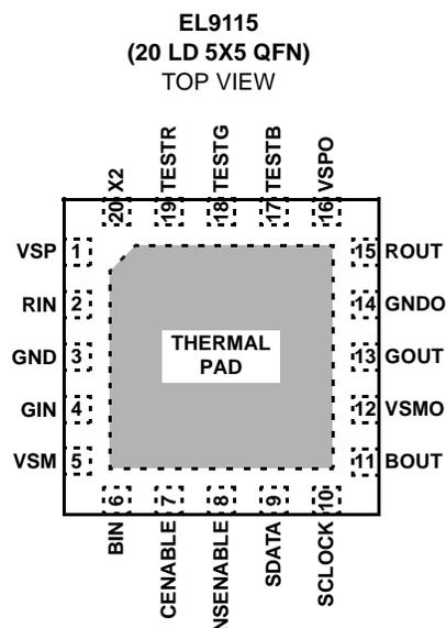
EXPOSED DIEPLATE SHOULD BE CONNECTED TO -5V
