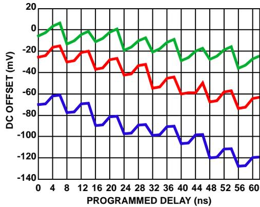
FIGURE 3. DC OFFSET vs DELAY TIME (GAIN = 2X)
