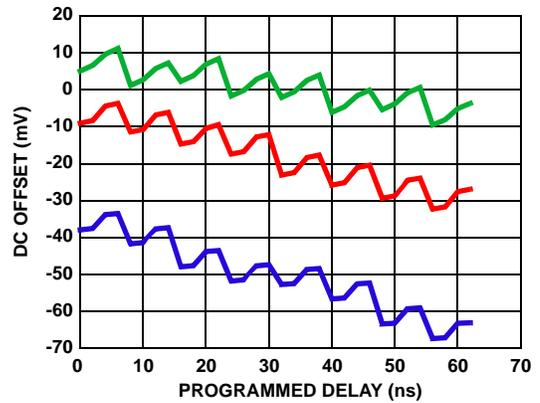
FIGURE 4. DC OFFSET vs DELAY TIME (GAIN = 1X)
