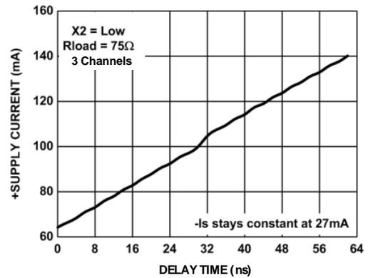
FIGURE 8. POSITIVE SUPPLY CURRENT vs DELAY TIME
