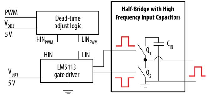
Figure 1: Block diagram of EPC9201/3 development board.
