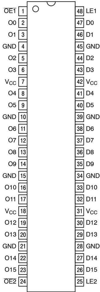
**Figure 1. Pinout: 48-Lead**
