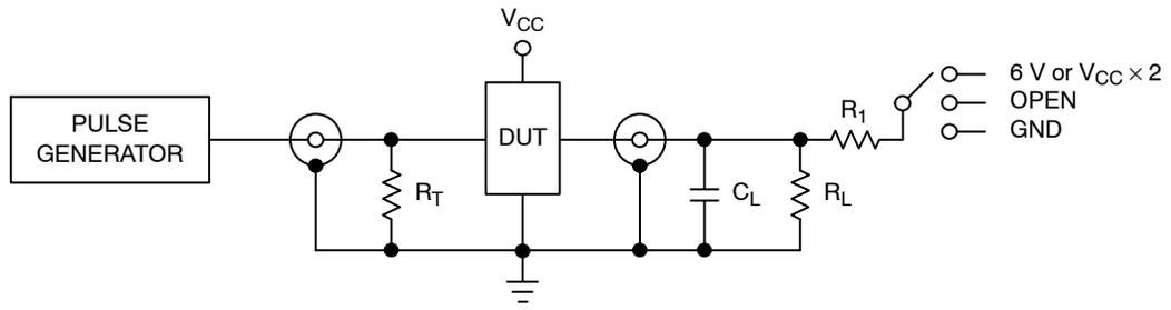
Figure 4. Test Circuit
