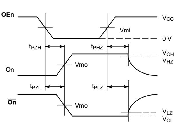
**WAVEFORM 2 - OUTPUT ENABLE AND DISABLE TIMES**
