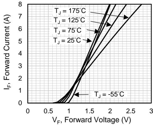
Fig.1 Forward Characteristics
