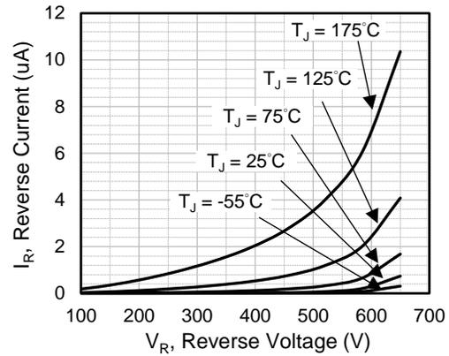
Fig.2 Reverse Characteristics
