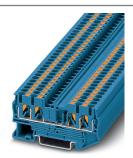
Feed-through terminal block, nom. voltage: 800 V, nominal current: 24 A, connection method: Push-in connection, number of connections: 4, cross section: 0.14 mm² - 4 mm², AWG: 26 - 12, width: 5.2 mm, height: 35.3 mm, color: blue, mounting type: NS 35/7,5, NS 35/15
