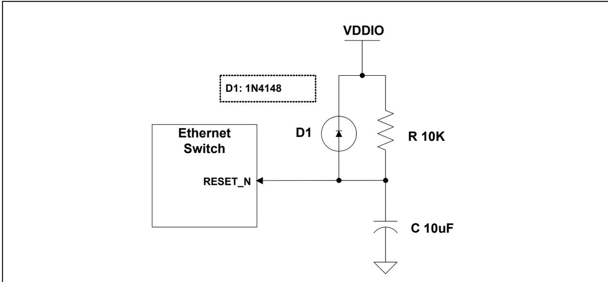
Figure 7-2 illustrates a reset circuit recommended for applications where reset is driven by another device, such as a CPU. At power-on reset, R, C and D1 provide the necessary ramp rise time to reset the KSZ9477S. The RST\_OUT\_N from the CPU provides a warm reset after power-up.
