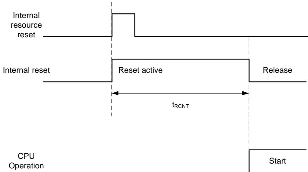
[1]: Internal resource reset is not included in return factor by the kind of Low-Power consumption mode.
