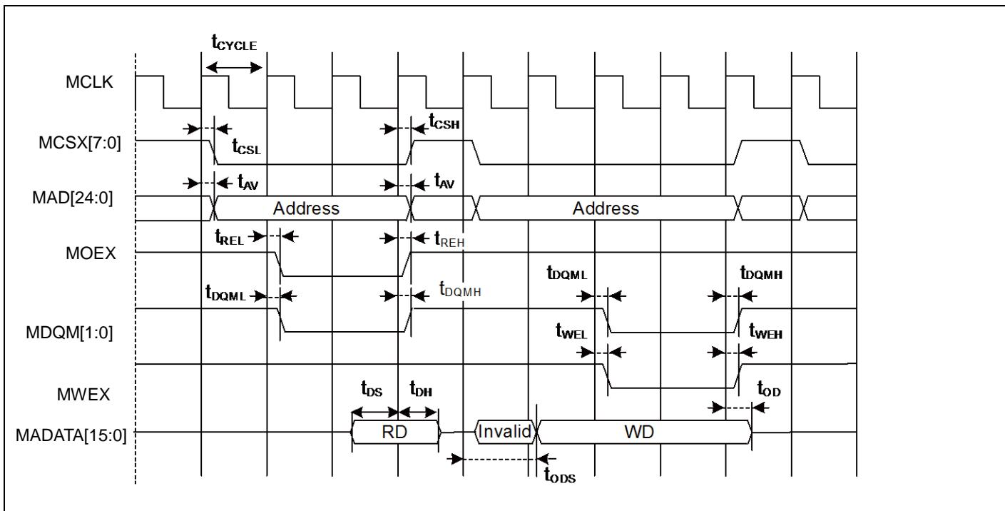
**Multiplexed Bus Access Asynchronous SRAM Mode**
