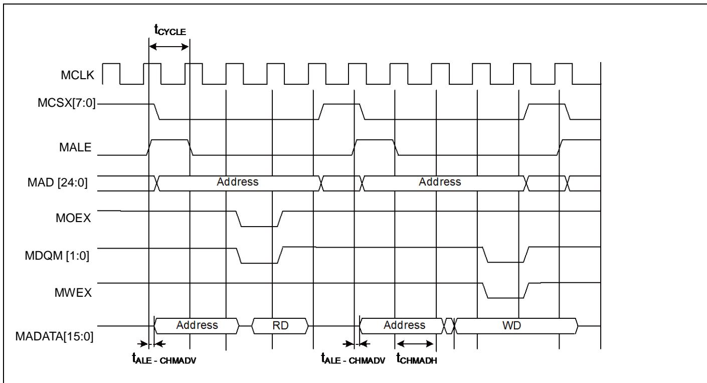
**Multiplexed Bus Access Synchronous SRAM Mode**
