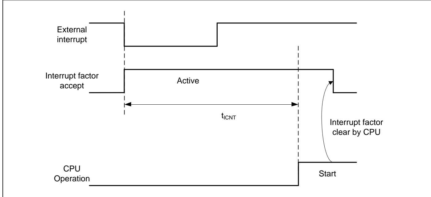
[1]: External interrupt is set to detecting fall edge.
