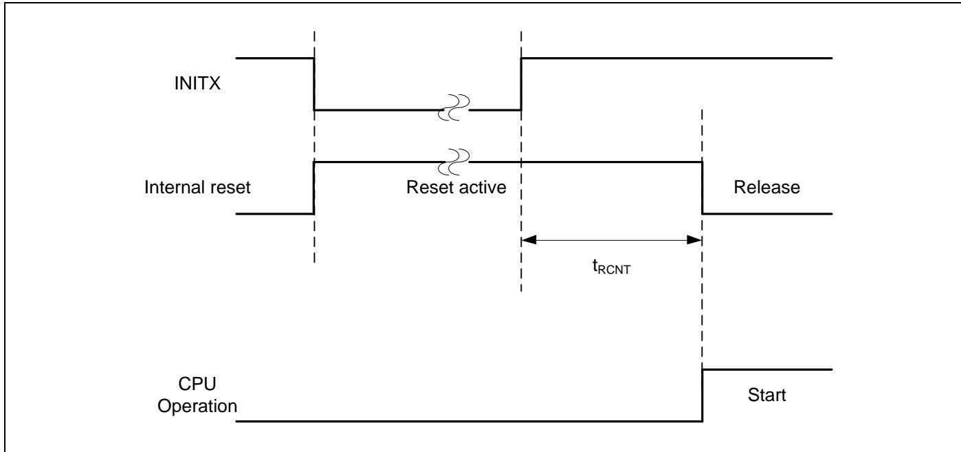
**Operation example of return from low power consumption mode (by internal resource reset<sup>[1]</sup>)**
