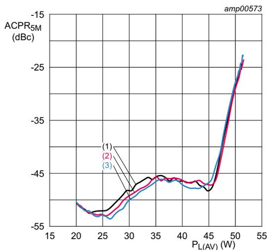
$V_{DS} = 48\text{ V}$ ;  $I_{Dq} = 1000\text{ mA}$ ; 46 % clipping.
