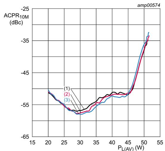
$V_{DS} = 48\text{ V}$ ;  $I_{Dq} = 1000\text{ mA}$ ; 46 % clipping.
