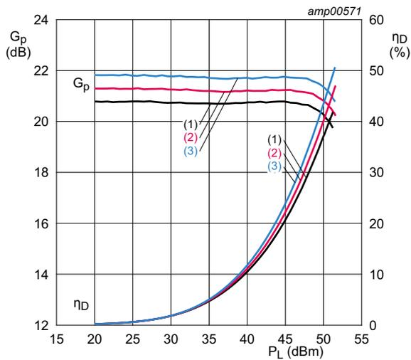
$V_{DS} = 48\text{ V}$ ;  $I_{Dq} = 1000\text{ mA}$ ; 46 % clipping.
