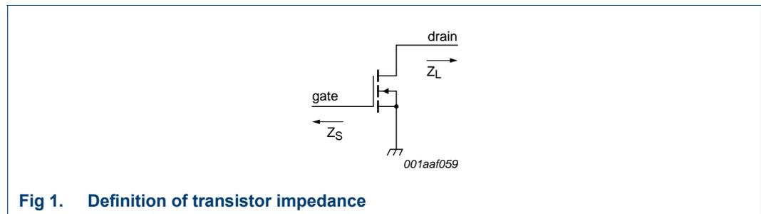
Fig 1. Definition of transistor impedance
