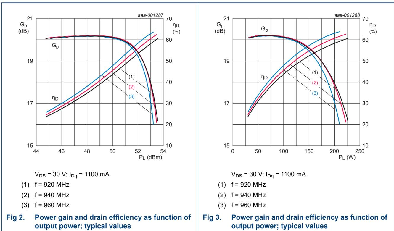
$V_{DS} = 30 \text{ V}$ ;  $I_{Dq} = 1100 \text{ mA}$ .
