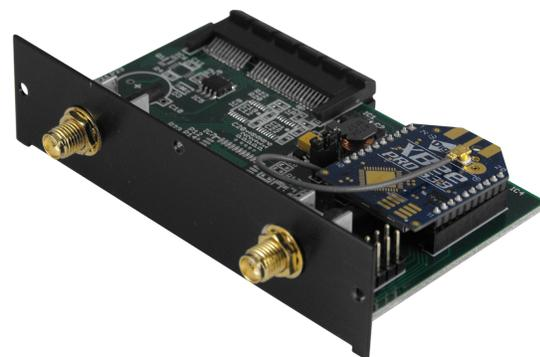
The new CloudGate M2M 3G gateway is certified on all major US cellular operators (CDMA/EV-DO and WADA/HSPA+) with global versions available. The MultiWireless peripheral board adds ZigBee®, Bluetooth® Low Energy and Wi-Fi capabilities to CloudGate.
