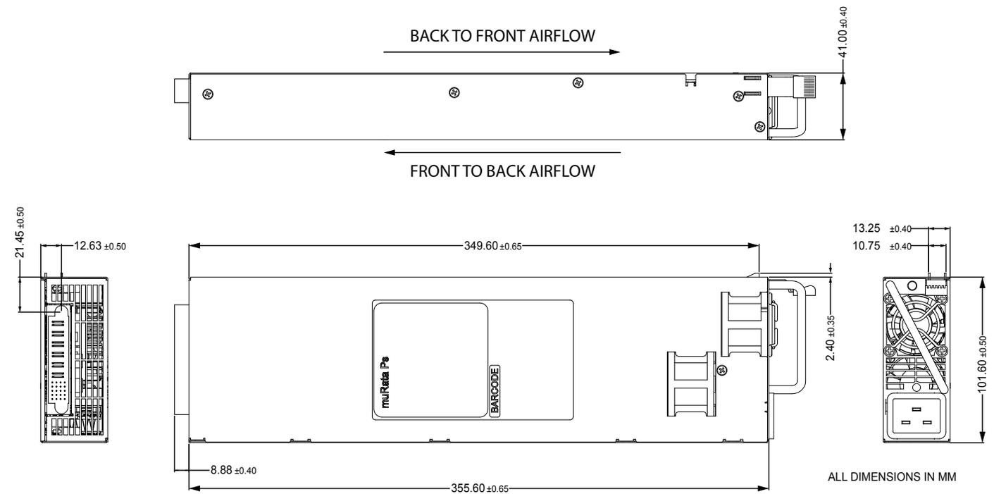
AC Input Connector/Inlet: IEC 60320-C20
