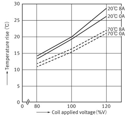
3-(1). Ambient temperature characteristics and coil applied voltage (TV-5 type)
