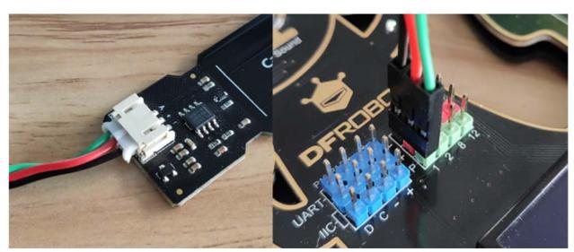
Programming to calibrate the soil sensor Download the program to micro: bit, according to the figure shown as below to obtain and record the reading in dry and in water. My data is 841 in dry, 543 in the water.
