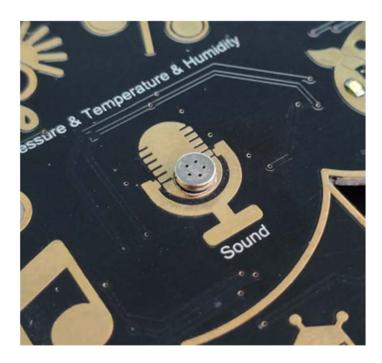
Here we can see a small sound sensor in the board which with a logo speaker. Small but sensitive, it can grasp the clapping, speaking sound and input the sound to micro: bit to calculate. Let's program to get the sound strength.
