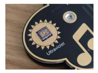
Ultraviolet sensor uses photosensitive elements to convert UV signals into electrical signals. It is only sensitive to ultraviolet light, insensitive to other lights like the usual sunlight, lamp light. So, we can measure the intensity of UV light more accurately. With the knowledge of UV sensors, let's measure the intensity of UV rays by programming.
