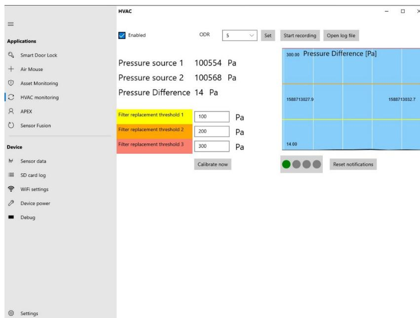
5. Observe the differential pressure change and filter replacement notification
