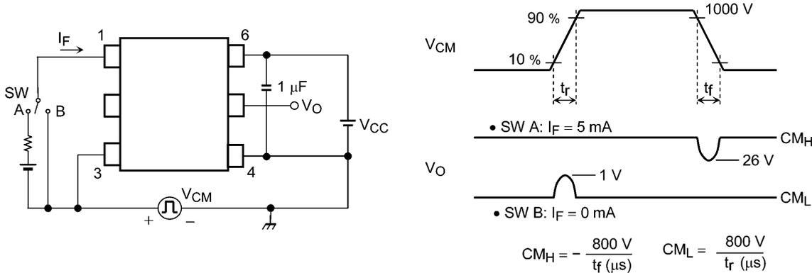
**Fig. 13.1.8 Common-Mode Transient Immunity Test Circuit and Waveform**
