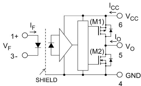
Note: A 1- $\mu$ F bypass capacitor must be connected between pin 6 and pin 4.
