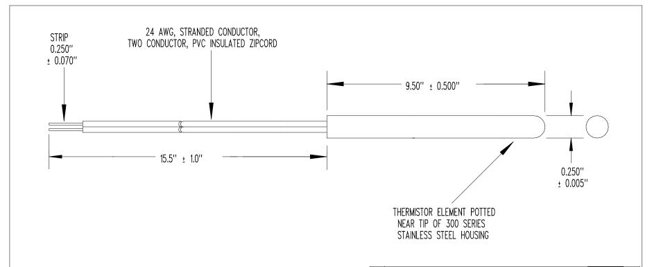
RESISTANCE @ +25'C = 100,000  $\Omega$  NOMINAL ACCURACY (0 TO +105'C) =  $\pm$  0.01'C OF R-T CHART SUPPLIED WITH PROBE RESISTANCE/TEMPERATURE CURVE = "J" BETA " $\beta$ " (0 TO +50'C) = 3,892'K NOMINAL TEMPERATURE COEFFICIENT @ +25'C = -4.4%/'C NOMINAL TYPICAL DRIFT: <0.01'C/YEAR MAXIMUM TEMPERATURE RATING = +105'C
