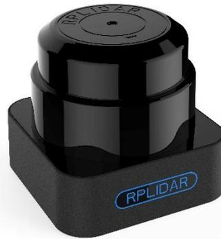
The RPLIDAR S1 is the next generation low cost 360 degree 2D laser scanner (LIDAR) solution developed by SLAMTEC. It can take up to 9200 samples of laser ranging per second with high rotation speed. And equipped with SLAMTEC patented OPTMAG technology, it breakouts the life limitation of traditional LIDAR system so as to work stably for a long time.
