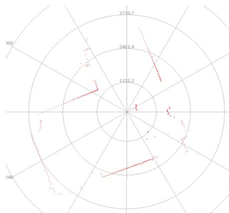
*Figure 1-3 The Obtained Environment Map from RPLIDAR S1 Scanning*
