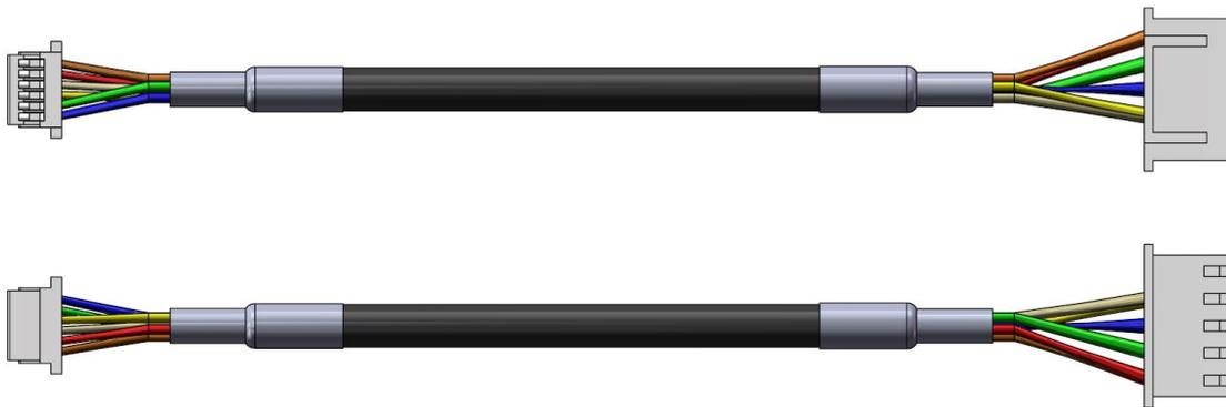
Figure 2-6 RPLIDAR S1 Interface Lead Schematic Diagram
