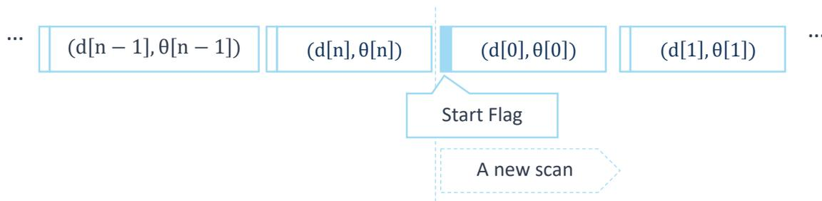
*Figure 1-5 The RPLIDAR S1 Sample Point Data Frames*
