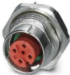
Bus system flush-type socket, with red contact carrier, 4-pos., M12 SPEEDCON, shielded, A-coded, rear/screw mounting with M16 thread, with straight solder connection
