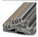
Double-level terminal block, Cross section: 0.14 mm<sup>2</sup> - 4 mm<sup>2</sup>, AWG: 26 - 12, Connection type: Push-in connection, Width: 5.2 mm, Color: gray, Mounting type: NS 35/7,5, NS 35/15
