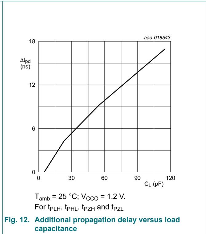
Fig. 12. Additional propagation delay versus load capacitance
