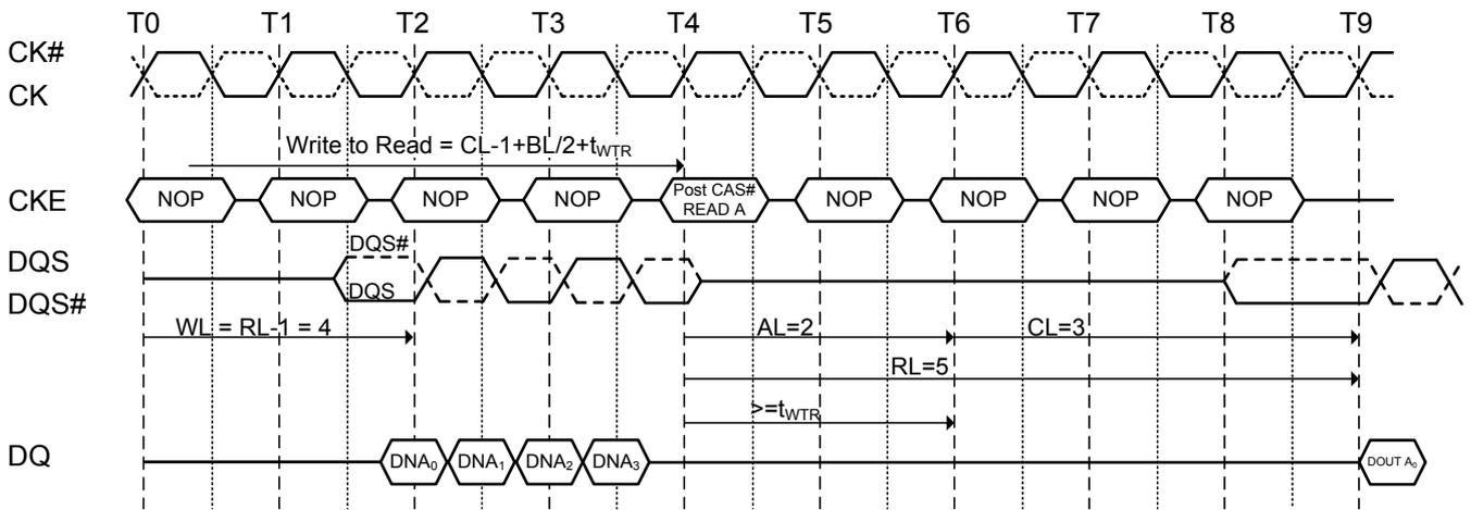
**NOTE :** The minimum number of clock from the burst write command to the burst read command is  $\lceil CL-1 + BL/2 + t_{WTR} \rceil$ . This  $t_{WTR}$  is not a write recovery time ( $t_{WR}$ ) but the time required to transfer the 4 bit write data from the input buffer into sense amplifiers in the array.  $t_{WTR}$  is defined in the timing parameter table of this standard.
