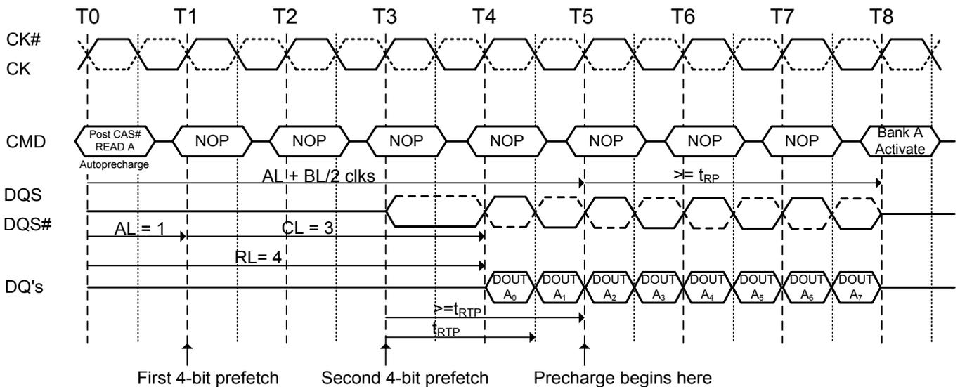
**Figure 38. Burst read operation with auto precharge:**
