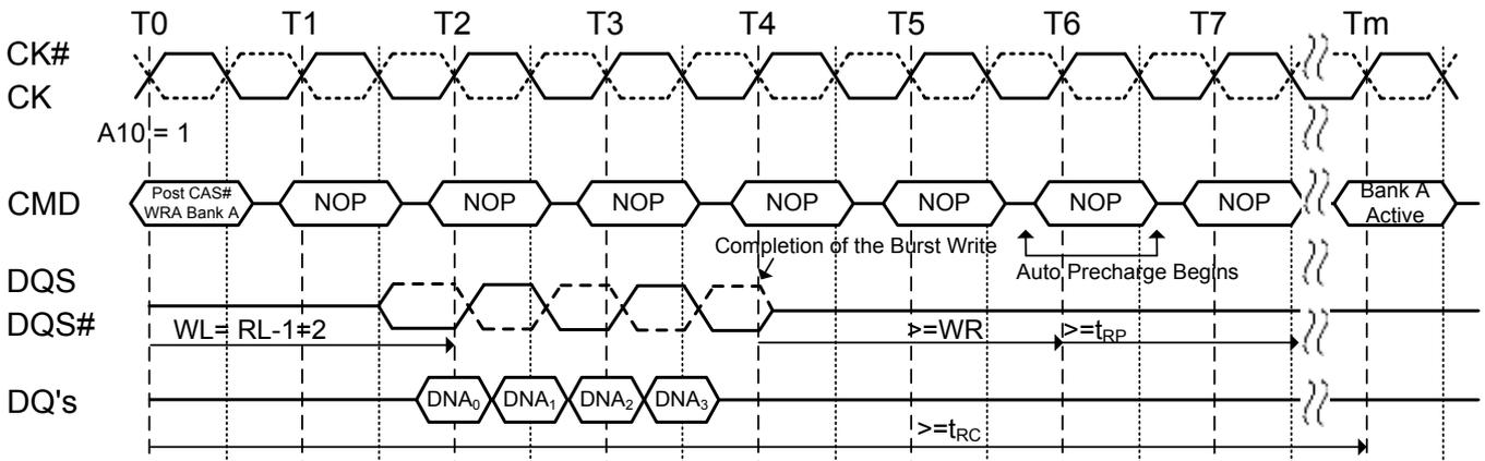
**Figure 42. Burst write with auto-precharge ( $WR+t_{RP}$ ):  $WL=4$ ,  $WR=2$ ,  $BL=4$ ,  $t_{RP}=3$**
