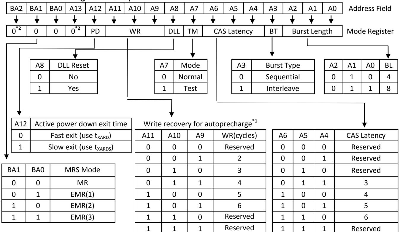
**NOTE 1:** For DDR2-800, WR min is determined by  $t_{CK}$  (avg) max and WR max is determined by  $t_{CK}$ (avg) min.  $WR [\text{cycles}] = RU \{t_{WR}[\text{ns}]/t_{CK}(\text{avg})[\text{ns}]\}$ , where RU stands for round up. The mode register must be programmed to this value. This is also used with  $t_{RP}$  to determine  $t_{DAL}$ .
