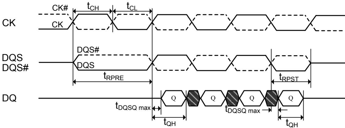
**Figure 18. Data input (write) timing**
