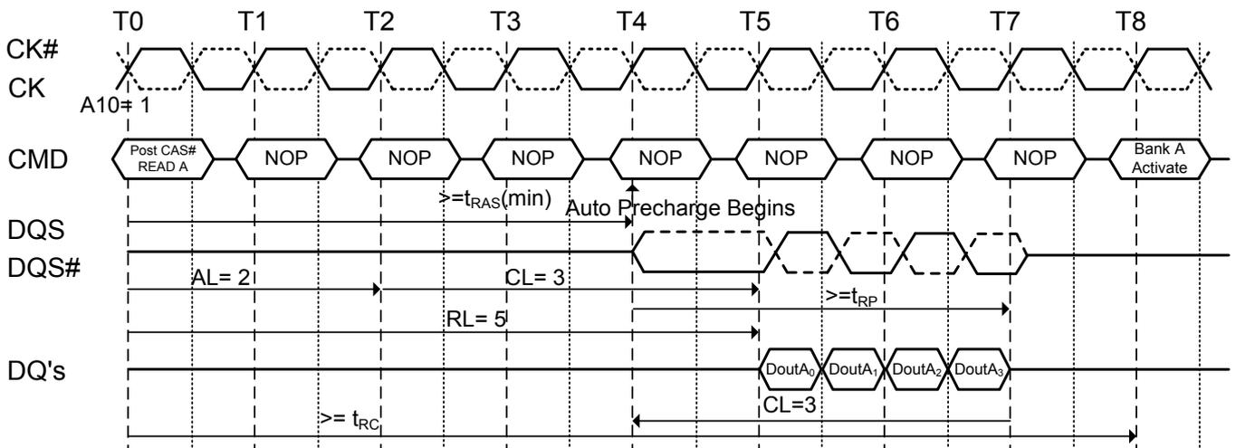
**Figure 40. Burst read operation with auto precharge followed by an activation to the same bank ( $t_{RP}$  Limit): (RL=5 (AL=2, CL=3, internal  $t_{RCD}$ =3, BL=4,  $t_{RTP} \leq 2$  clocks)**
