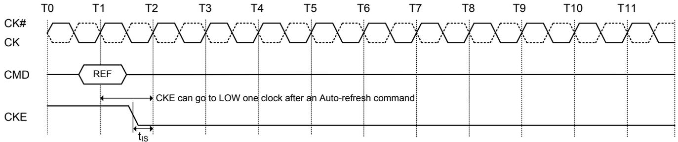
**Figure 53. Active command to power-down entry**
