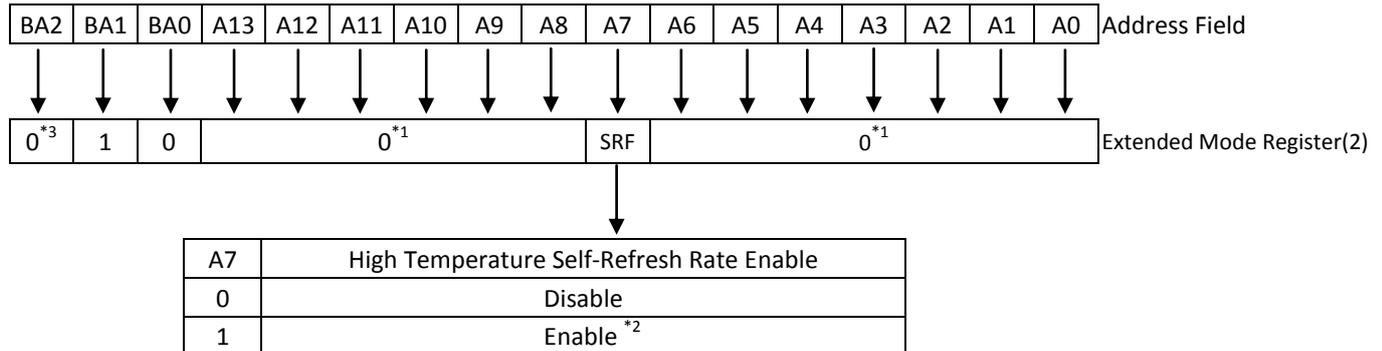
**NOTE 1:** The rest bits in EMRS(2) are reserved for future use and all bits in EMRS(2) except A7, BA0 and BA1 must be programmed to 0 when setting the extended mode register(2) during initialization.
