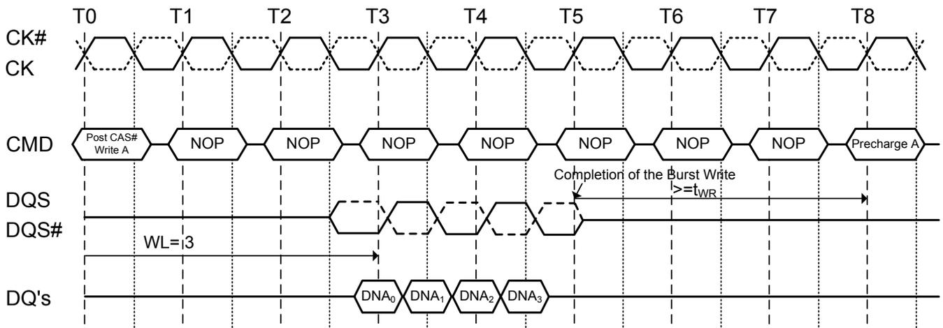
**Figure 36. Burst write followed by precharge: WL= (RL-1) =4**
