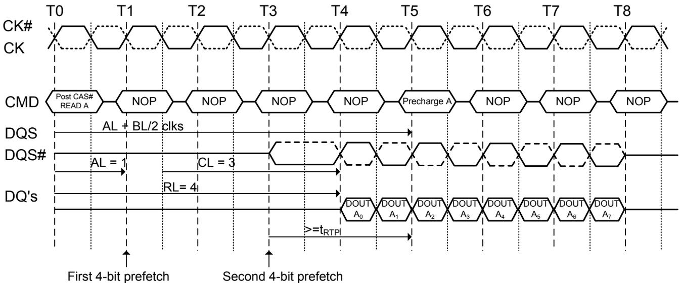
**Figure 32. Burst read operation followed by precharge:**
