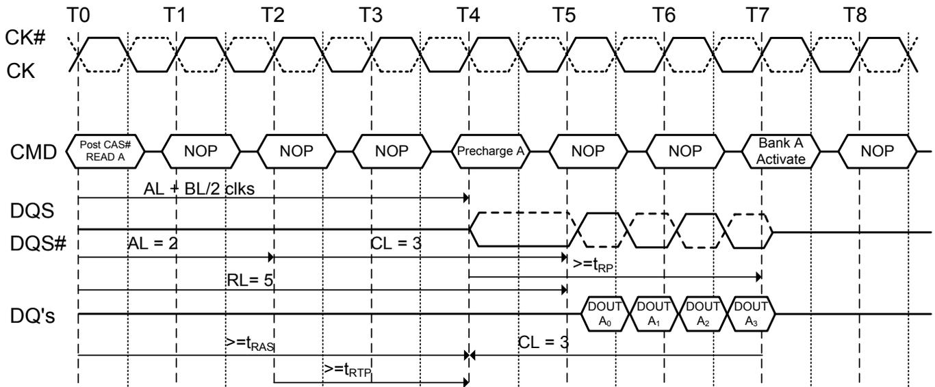
**Figure 33. Burst read operation followed by precharge:**
