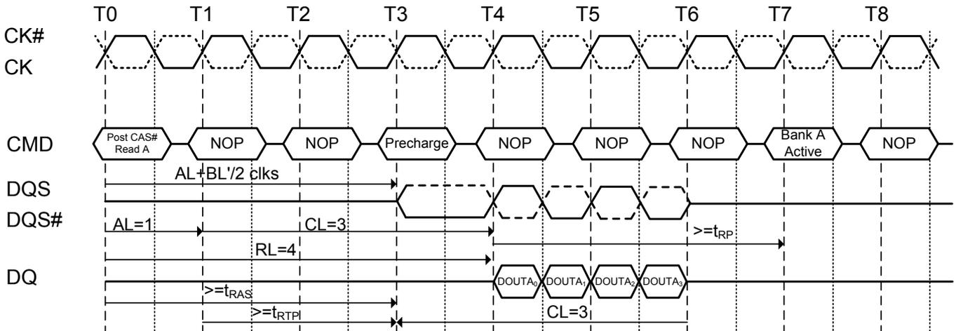
**Figure 31. Burst read operation followed by precharge:**
