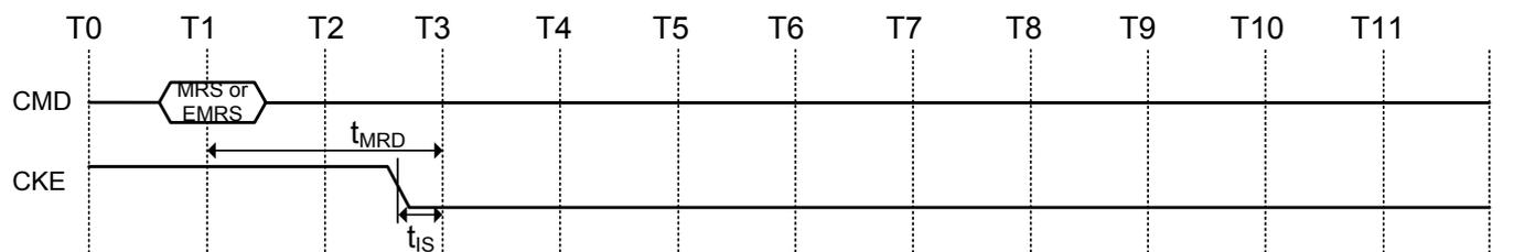
**Figure 56. Asynchronous CKE LOW event**
