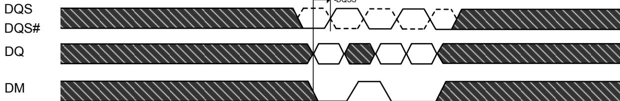
**Figure 30. Burst read operation followed by precharge:**
