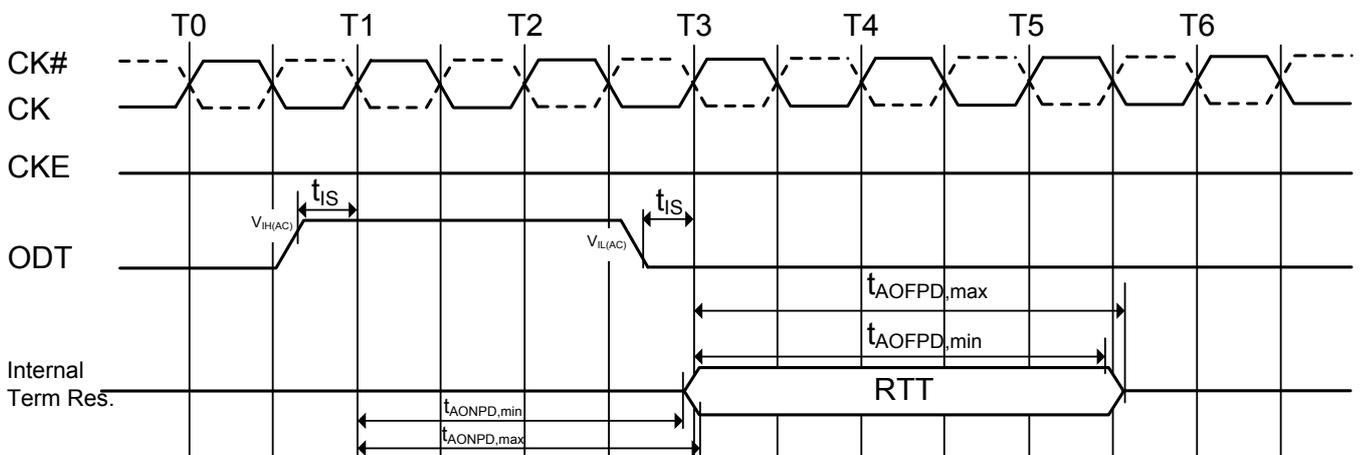
**Figure 13. ODT timing mode switch at exit power-down mode**
