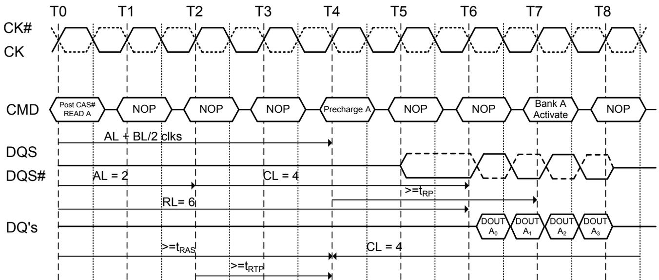
**Figure 34. Burst read operation followed by precharge:**
