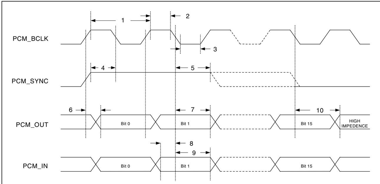
Figure 20: PCM (Long Frame Sync, Slave Mode) Timing
