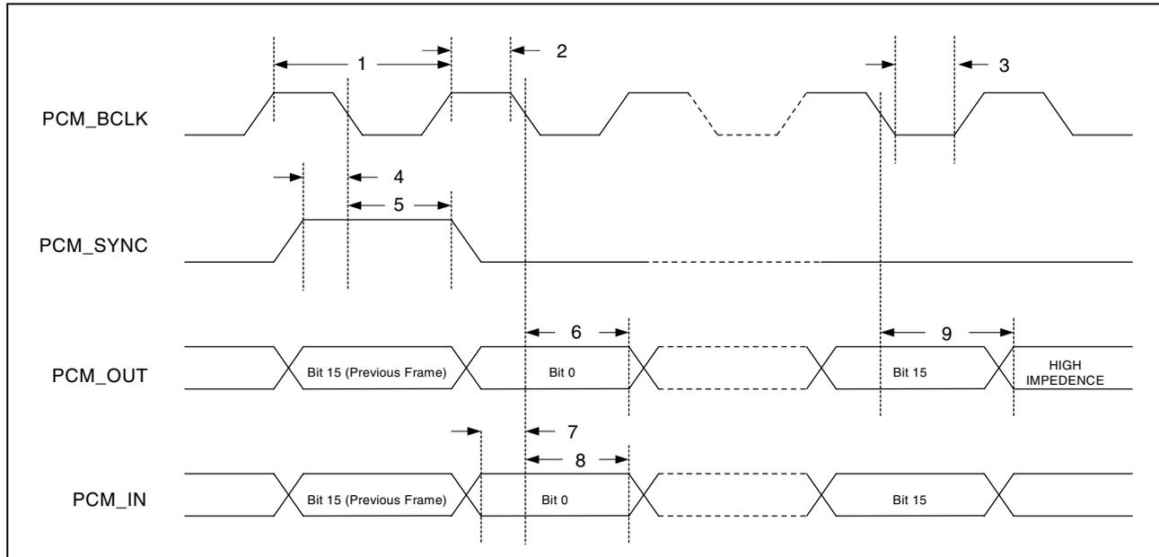
Figure 18: PCM (Short Frame Sync, Slave Mode) Timing
