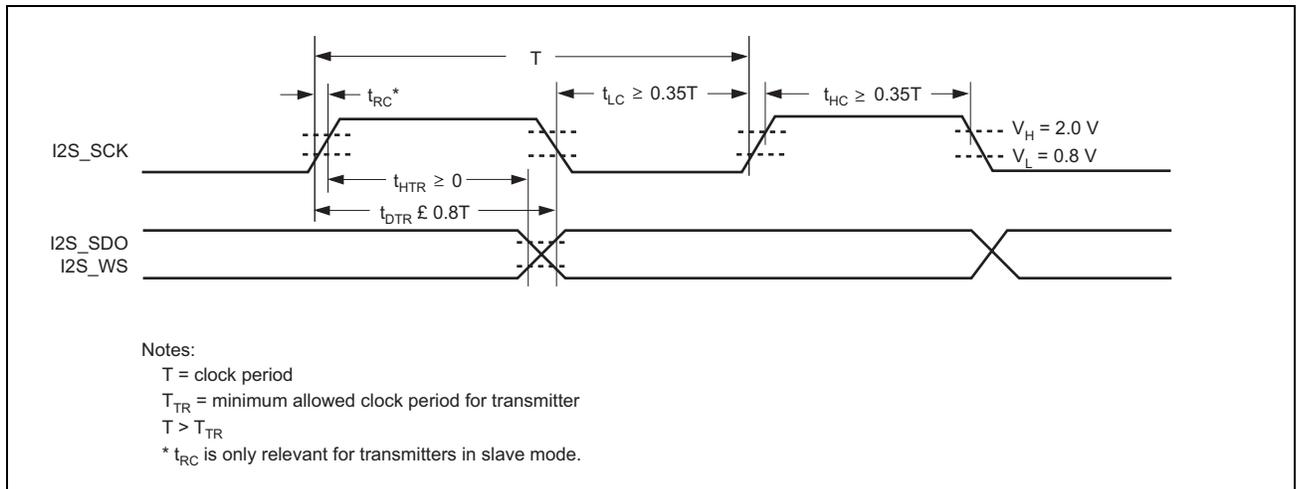
**Figure 21: I<sup>2</sup>S Transmitter Timing**
