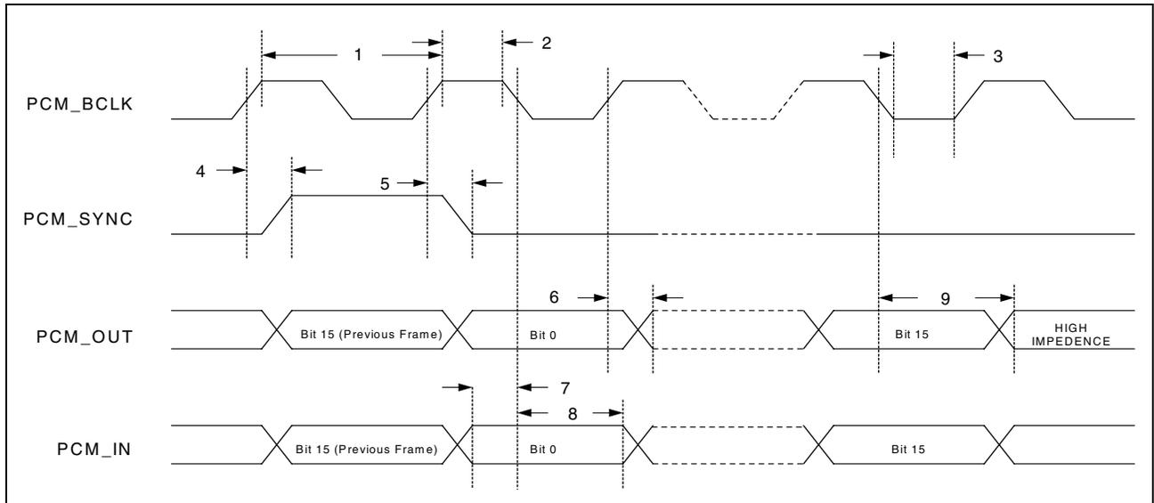
Figure 17: PCM (Short Frame Sync, Master Mode) Timing
