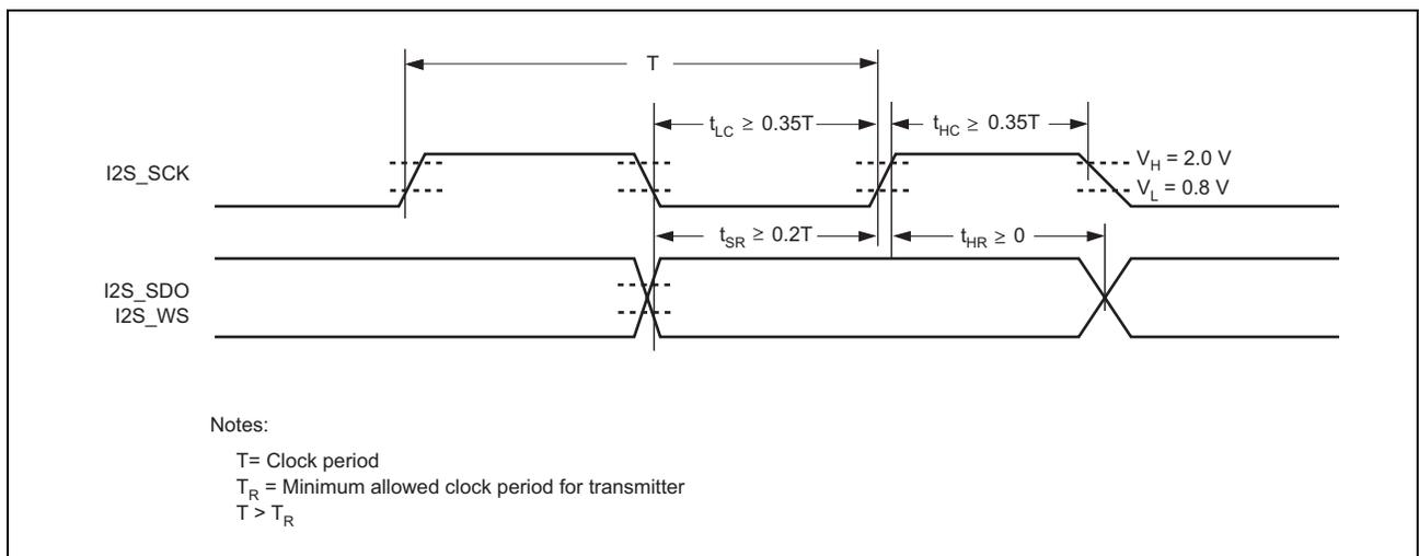
**Figure 22: I<sup>2</sup>S Receiver Timing**
