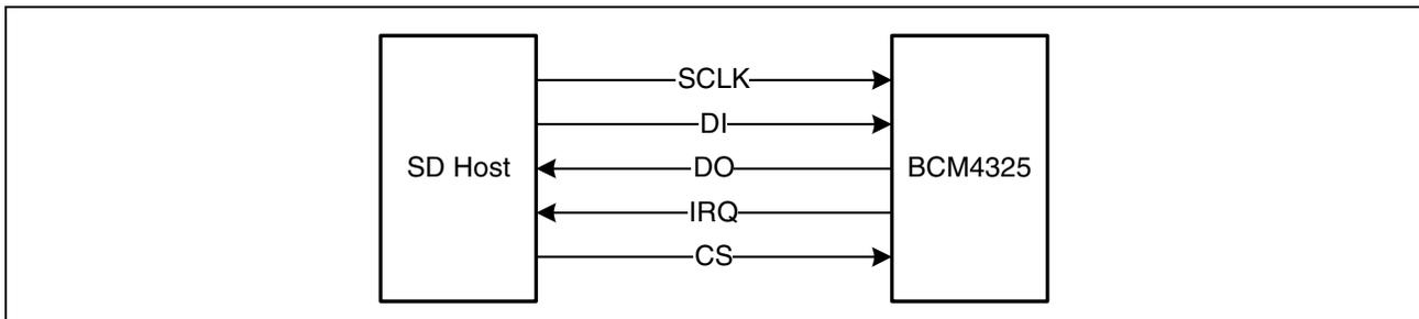
Figure 15: Signal Connections to SDIO Card (SPI Mode)
