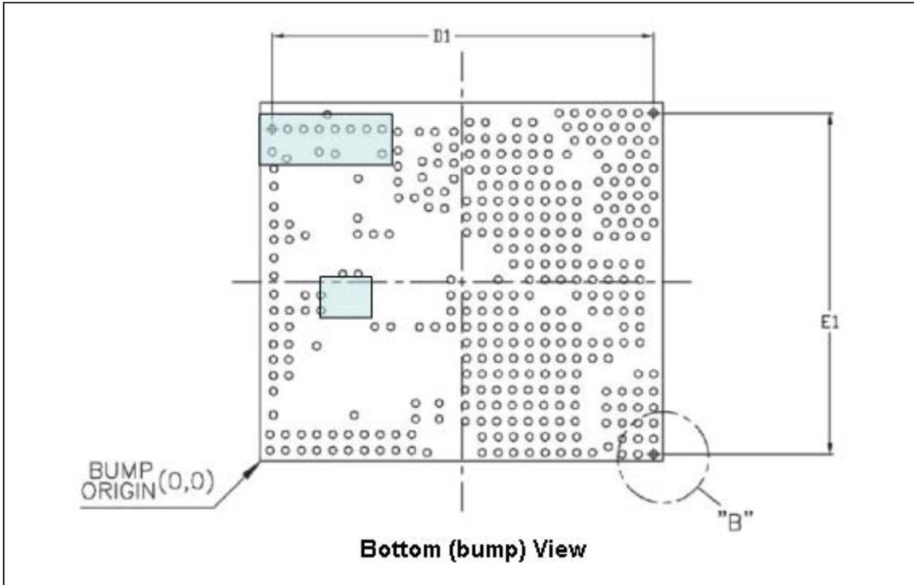
Figure 38: WLAN Section Second Metal Keepout Area
