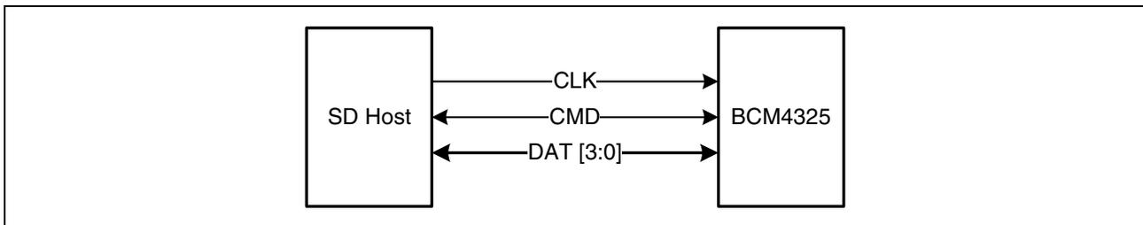
Figure 13: Signal Connections to SDIO Card (SD 4-Bit Mode)
