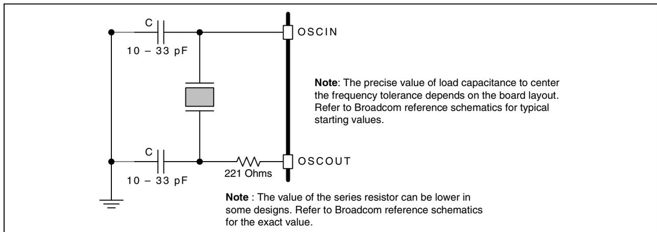
Figure 6: Recommended Oscillator Configuration
