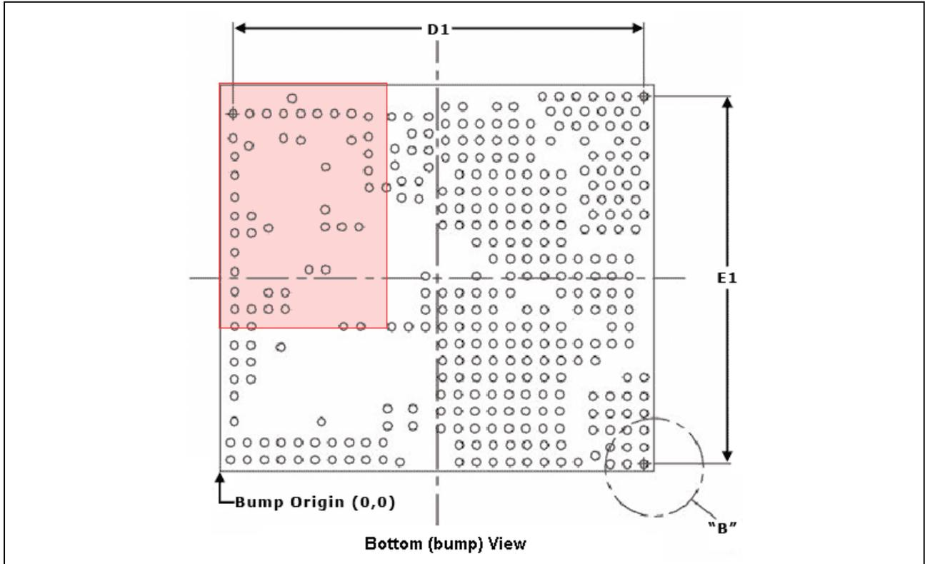
Figure 37: WLAN Section Top Metal Keepout Area
