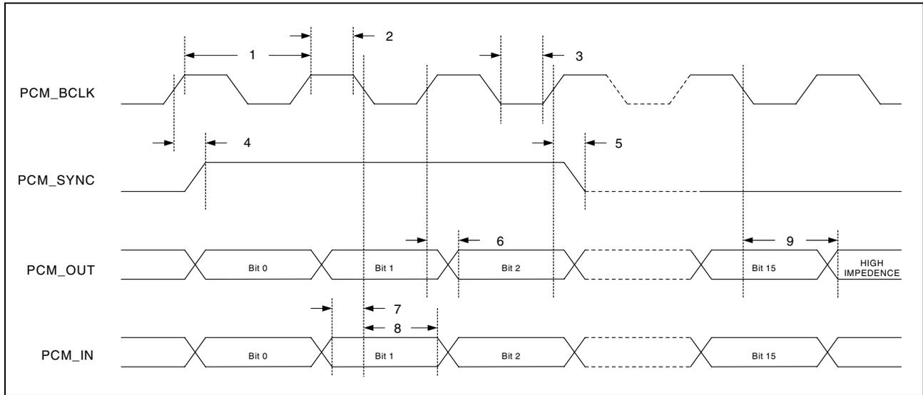
Figure 19: PCM (Long Frame Sync, Master Mode) Timing
