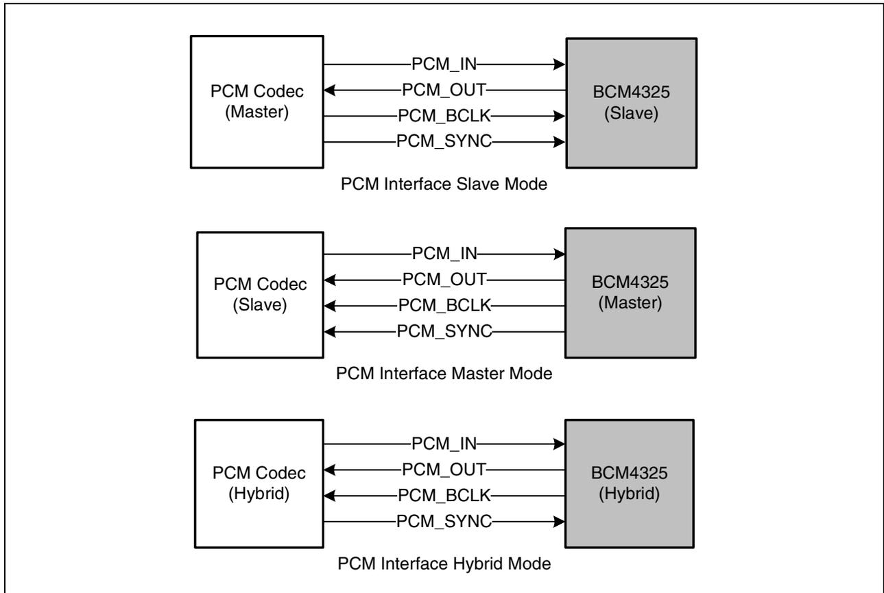
Figure 8: PCM Interface with Linear PCM Codec
