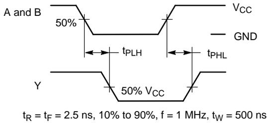
**Figure 3. Switching Waveforms**
